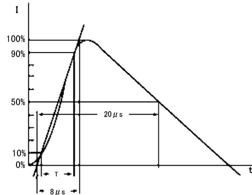
Fig. 6.3.2 Based on IEC61000-4-5 8/20  $\mu$ s pulse.
