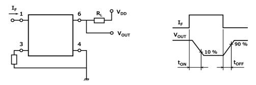
Fig. 15.1 Switching Time Test Circuit and Waveform
