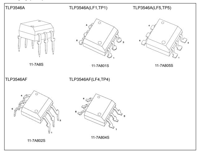
Note: Through-hole type: TLP3546A, TLP3546AF Lead forming option: (LF1), (LF4), (LF5) Taping option: (TP1), (TP4), (TP5)
