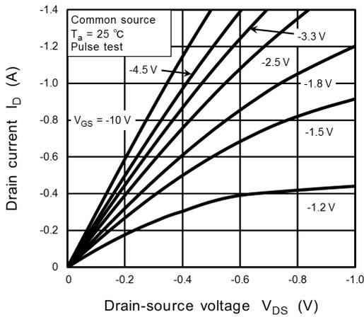
**Fig. 8.1  $I_D - V_{DS}$**
