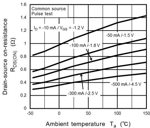
**Fig. 8.5  $R_{DS(ON)} - T_a$**
