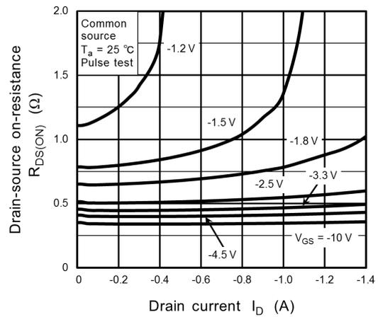
**Fig. 8.4  $R_{DS(ON)} - I_D$**
