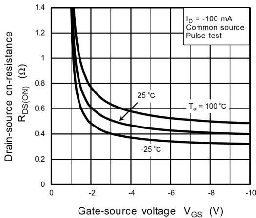
**Fig. 8.3  $R_{DS(ON)} - V_{GS}$**
