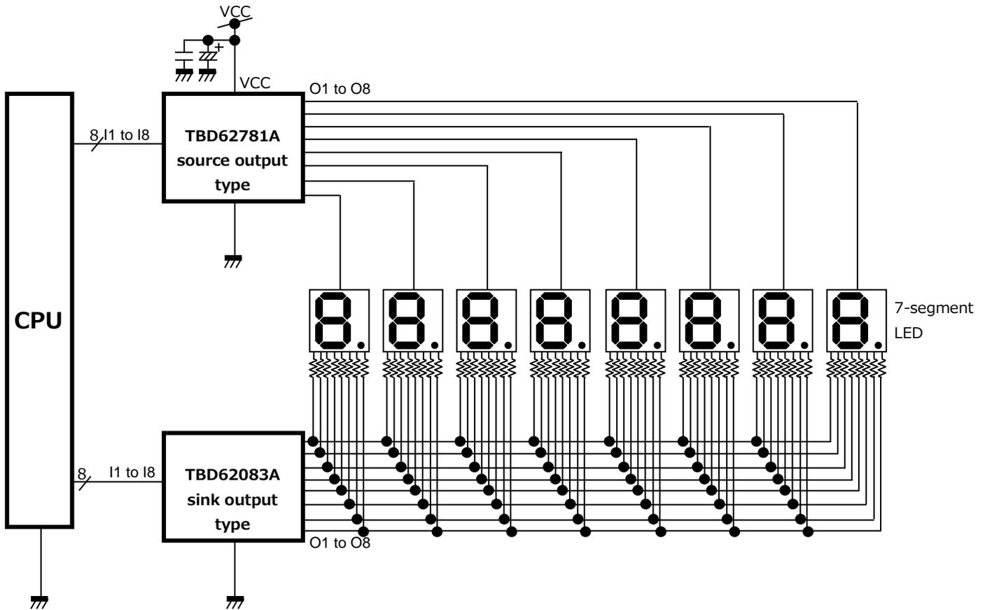
For voltage stabilization and noise rejection, please connect a stacked ceramic capacitor (0.01  $\mu\text{F}$  to 1  $\mu\text{F}$ ) or an electrolytic capacitor (10  $\mu\text{F}$  to 100  $\mu\text{F}$ ) to VCC line. The capacitor is recommended to be connected as close to the IC as possible.
