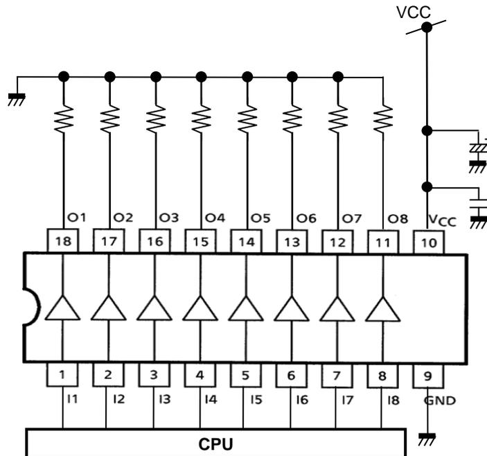
For voltage stabilization and noise rejection, please connect a stacked ceramic capacitor (0.01  $\mu\text{F}$  to 1 $\mu\text{F}$ ) or an electrolytic capacitor (10  $\mu\text{F}$  to 100  $\mu\text{F}$ ) to VCC line. The capacitor is recommended to be connected as close to the IC as possible.
