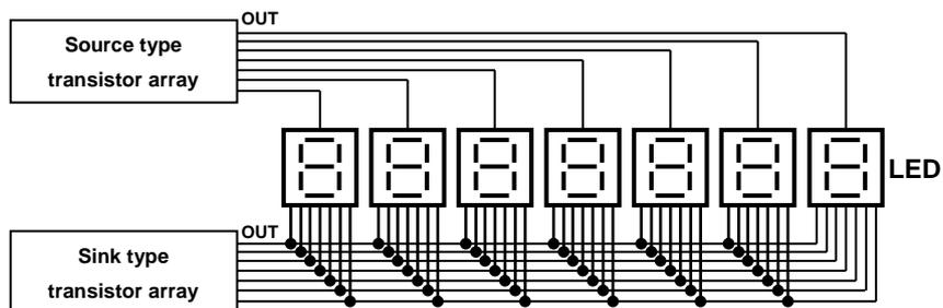
●Construction of output circuit
