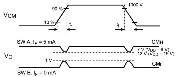
$$CM_H = - \frac{800 \text{ (V)}}{t_f \text{ (}\mu\text{s)}} \quad CM_L = \frac{800 \text{ (V)}}{t_r \text{ (}\mu\text{s)}}$$
