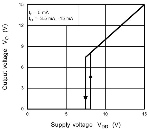
**Fig. 12.2.11**  $V_O - V_{DD}$
