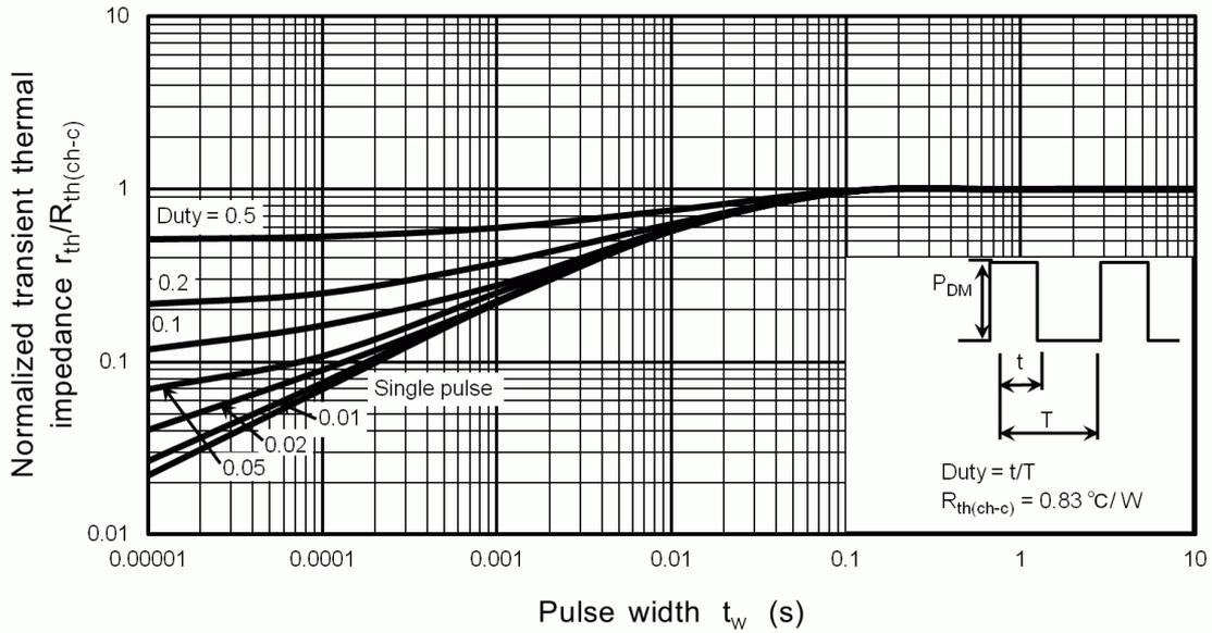
**Fig. 8.15**  $r_{th}/R_{th(ch-c)} - t_w$
