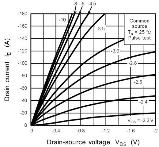
Fig. 8.2  $I_D - V_{DS}$
