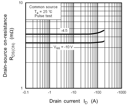
**Fig. 8.8  $R_{DS(ON)} - I_D$**
