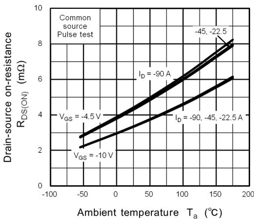
**Fig. 8.9  $R_{DS(ON)} - T_a$**
