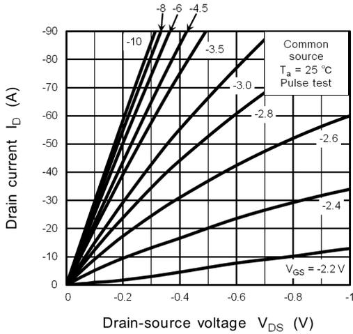
Fig. 8.1  $I_D - V_{DS}$
