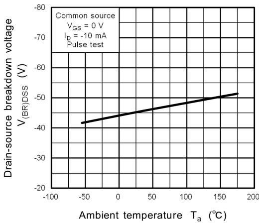
**Fig. 8.11  $V_{(BR)DSS} - T_a$**
