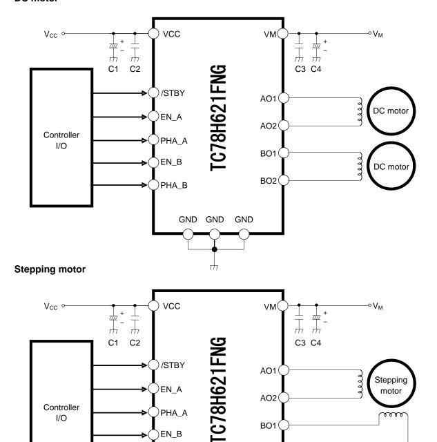
All the grounding wires of the device must run on the solder mask on the PCB and be externally terminated at only one point.
