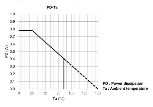
When mounted on a glass epoxy board (50 mm × 50 mm × 1.6 mm, Cu area: 40 %, Cu thick: 35 µm)
