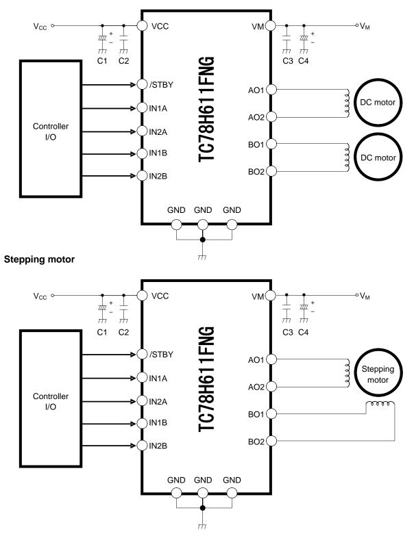
All the grounding wires of the device must run on the solder mask on the PCB and be externally terminated at only one point.
