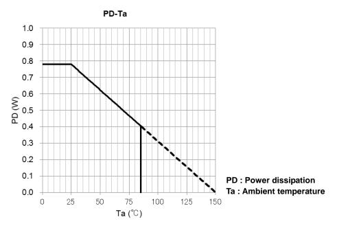
When mounted on a glass epoxy board (50 mm  $\times$  50 mm  $\times$  1.6 mm, Cu area: 40 %, Cu thick: 35 µm)
