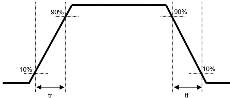
**Figure 6.1 Switching characteristics**
