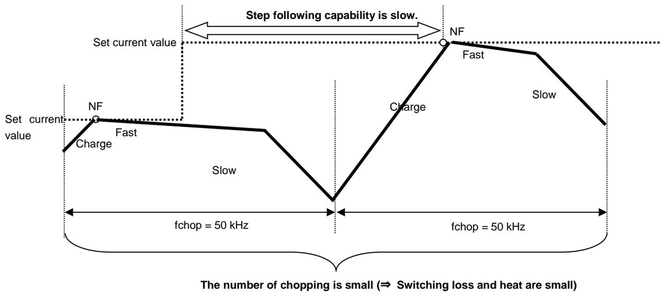
**Figure 4.3 Chopping frequency (50 kHz)**
