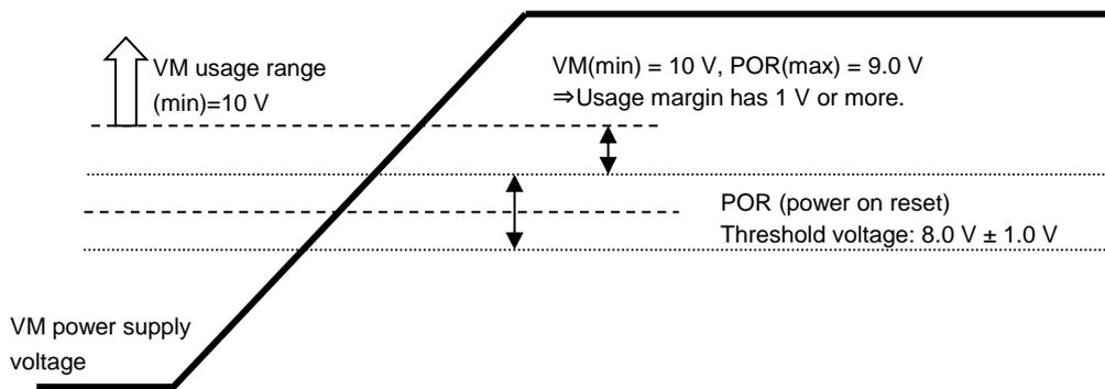
Figure 1.1 Power supply voltage and usage range
