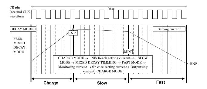
Figure 5.1 Mixed Decay waveform
