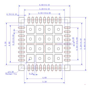
Figure 11.1 QFN36 foot pattern
