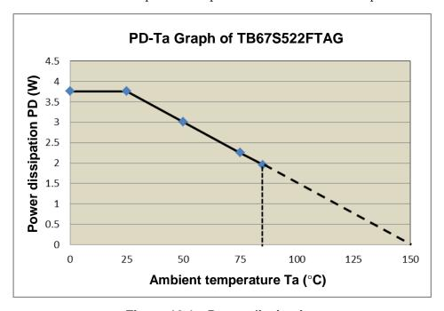
Figure 10.1 Power dissipation
