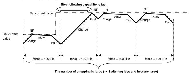
Figure 4.2 Chopping frequency (100 kHz)
