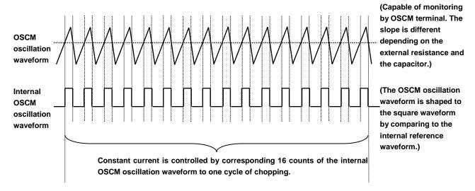
Figure 4.1 OSCM oscillation frequency
