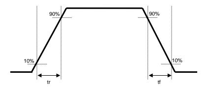
Figure 6.1 Switching characteristics
