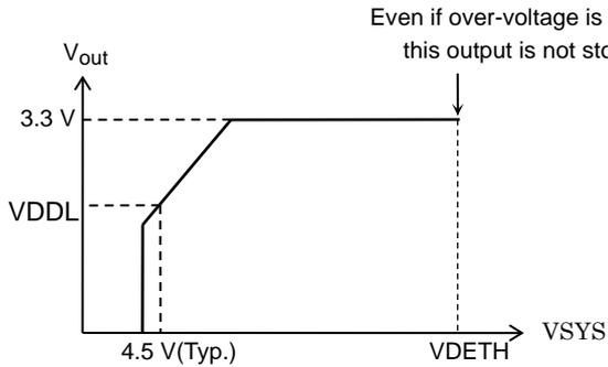
VDD output voltage - Load characteristics
