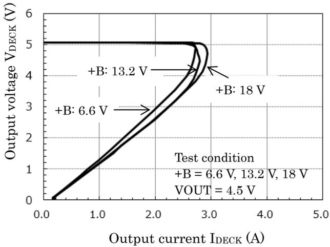
$V_{DECK}-I_{DECK}$  (8.5 V setting)
