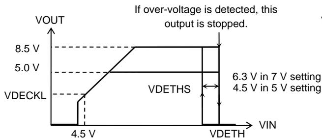
Load characteristics in DECK 7.0 V / 5.0 V setting
