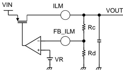
$$V_{OUT} = V_R \times (R_c + R_d) / R_d \quad V_R = 0.8 \text{ V (Typ.)}$$
