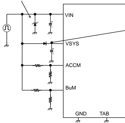
Inserting a diode to VSYS pin enables the reverse current prevention from VDD pin at +B momentary disconnection.
