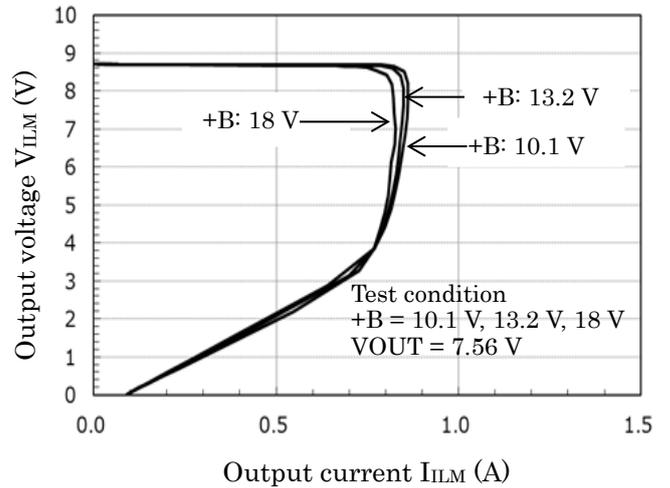
$V_{DECK}-I_{DECK}$  (5 V setting)
