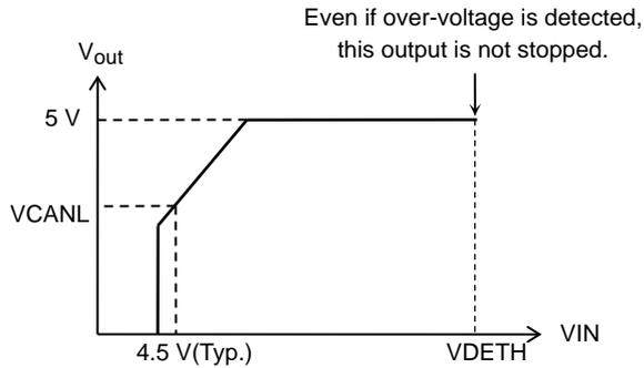
CAN output voltage - Load characteristics
