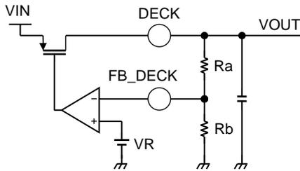
$$V_{OUT} = V_R \times (R_a + R_b) / R_b \quad V_R = 0.8 \text{ V (Typ.)}$$
