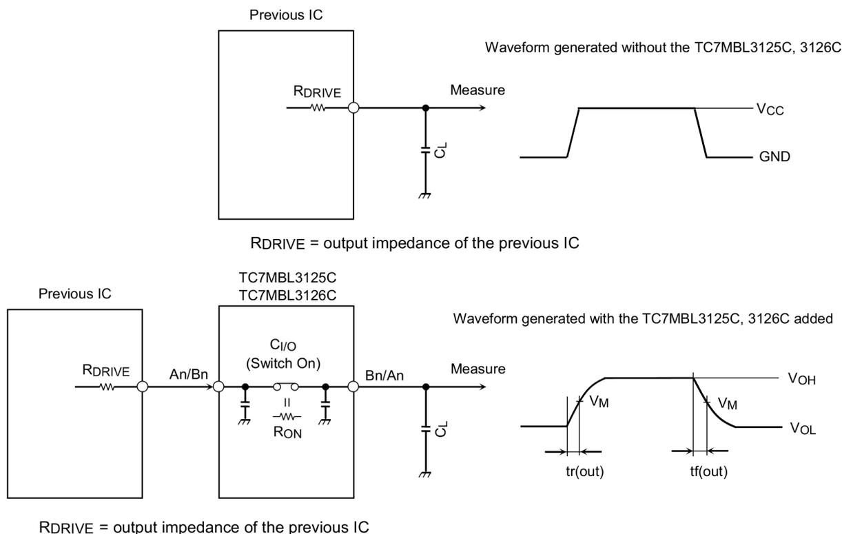
**Fig. 12.1 Calculation Circuit**
