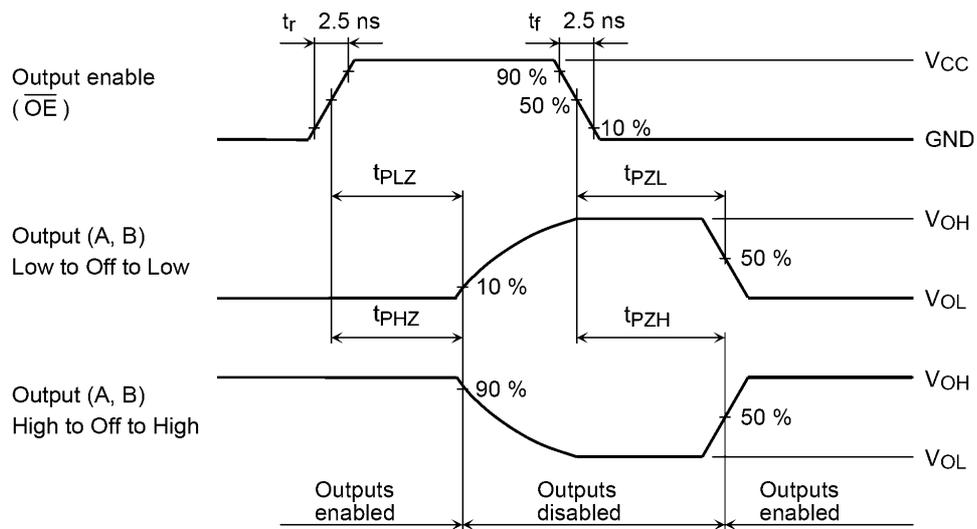
**Fig. 11.5.1 AC Waveform  $t_{PLZ}$ ,  $t_{PHZ}$ ,  $t_{PZL}$ ,  $t_{PZH}$**
