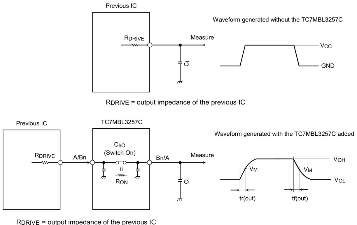
**Fig. 12.1 Calculation Circuit**
