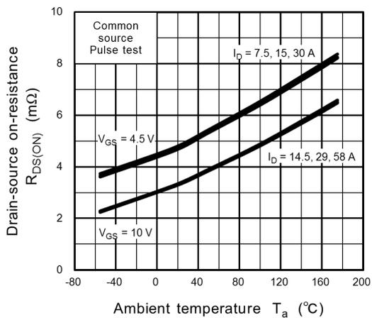
**Fig. 8.9**  $R_{DS(ON)} - T_a$
