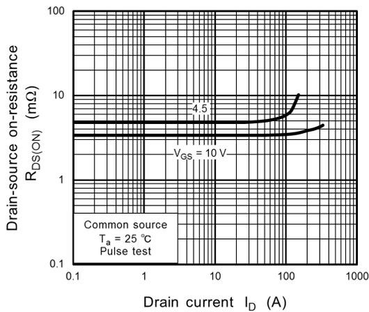
Fig. 8.5  $R_{DS(ON)} - I_D$
