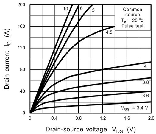
Fig. 8.2  $I_D - V_{DS}$
