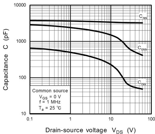
**Fig. 8.11** Capacitance -  $V_{DS}$
