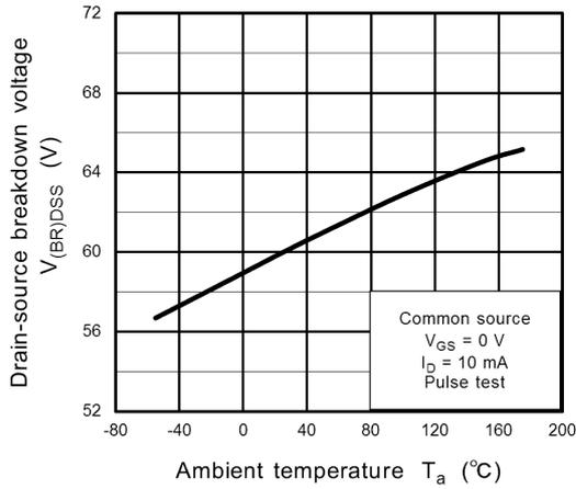
**Fig. 8.7**  $V_{(BR)DSS} - T_a$
