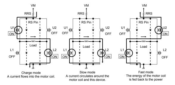
**Output transistor operational function**
