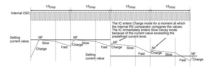
The Charge period starts as the internal oscillator clock starts counting. When the output current reaches the predefined current level, the internal RS comparator detects the predefined current level (NF); as a result, the IC enters Slow Decay mode.
