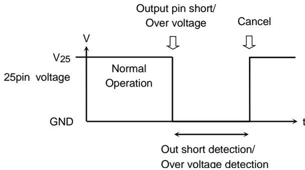
**Figure 9 Output short detection/Overvoltage detection**
