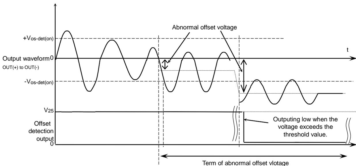
Figure 8 Output waveform of amplifier and pin25
