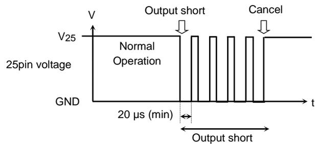
**Figure10 Output to Output short detection**
