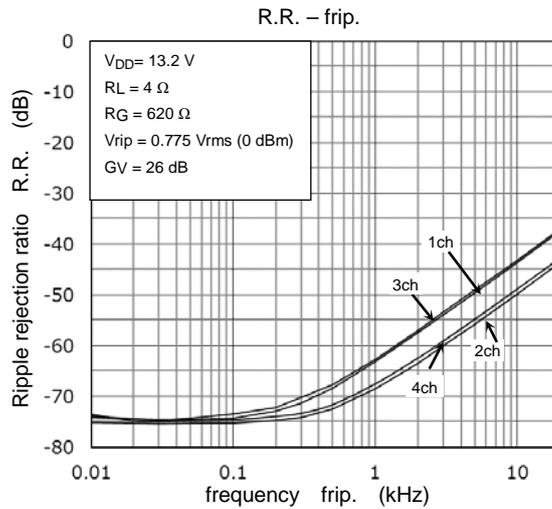
Figure 13-5 Frequency Characteristics of Ripple Rejection Rate
