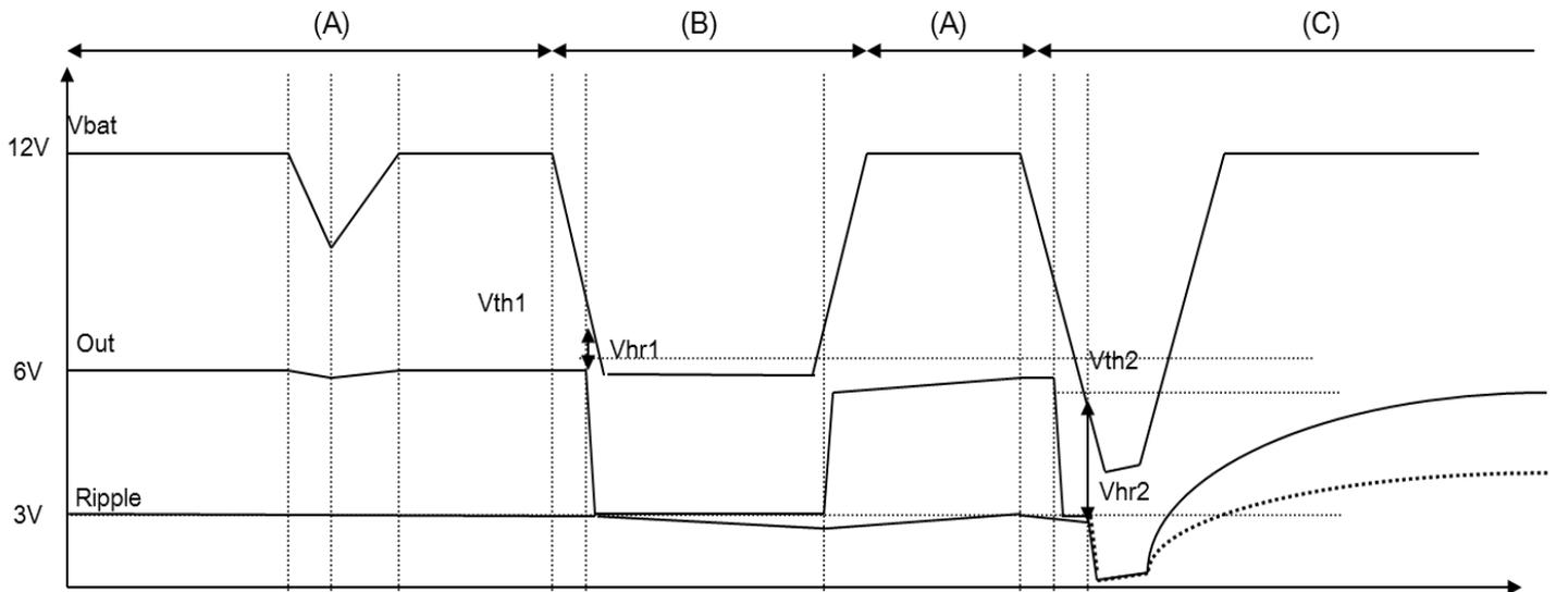
Figure 12 Output  $V_{DD}/2$  voltage in lowering  $V_{DD}$
