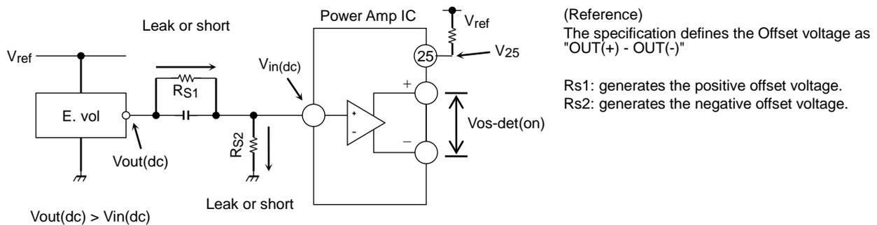
Figure 7 Generating example of abnormal output offset voltage
