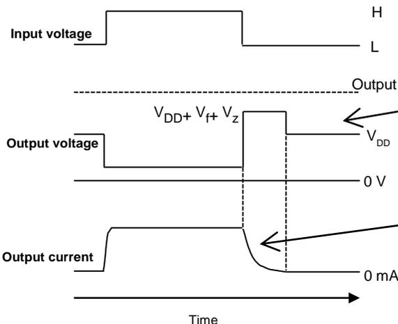
When the current fall time from ON to OFF degrades, connecting the zener diode to the COMMON pin is effective.
