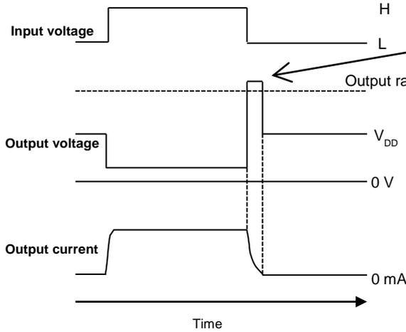
In case of driving inductive loads, the voltage might exceed the output rating at ON/OFF switching. It is occurred by the influence of the counter electromotive force.
