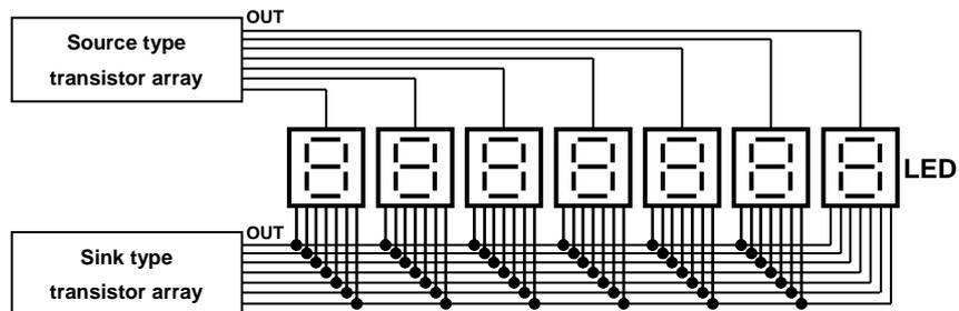
• Construction of output circuit
