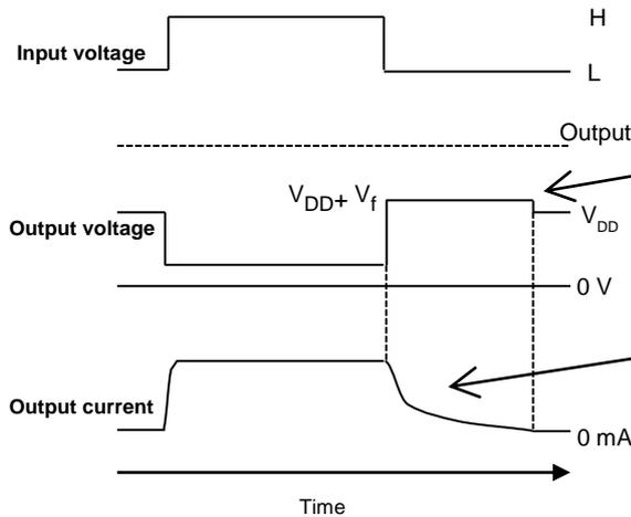
Generation of the counter electromotive force can be prevented by discharging through a clamp diode in the IC.
