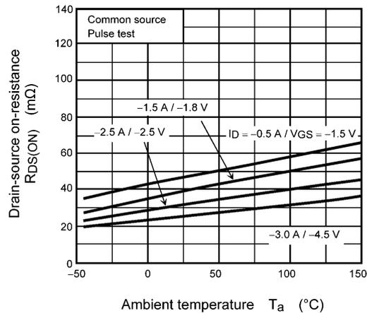
Fig. 7.6  $R_{DS(ON)} - T_a$
