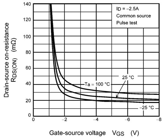
Fig. 7.4  $R_{DS(ON)} - V_{GS}$
