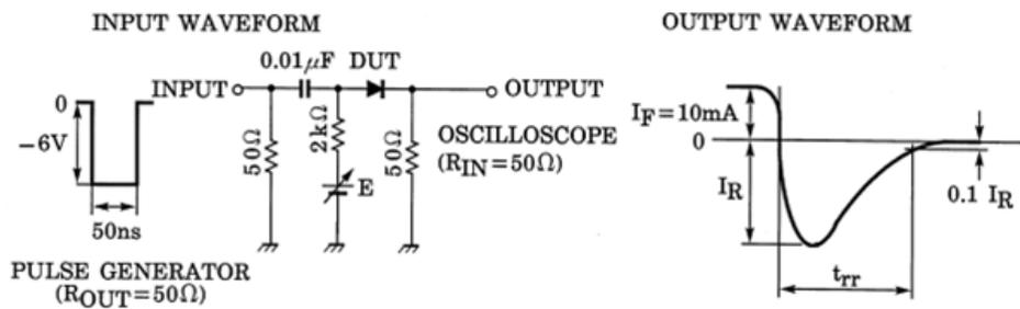
**Fig. 4.1 Reverse recovery time ( $t_{rr}$ ) Test circuit**
