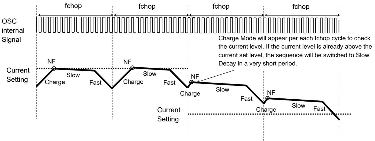
**Figure 6.16 When the next current step is lower**
