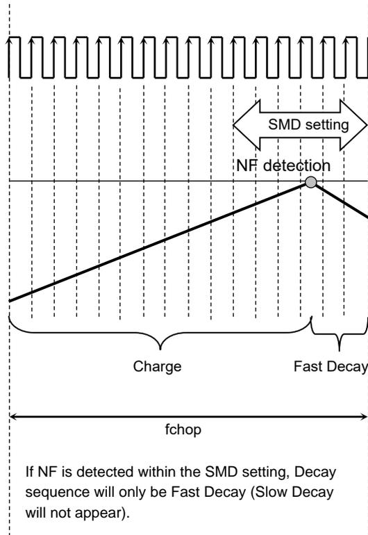
**Figure 6.13 Constant current PWM function and timings (3)**
