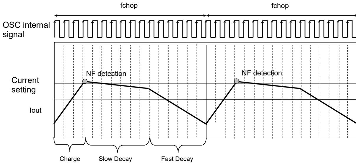
**Figure 6.10 Mixed Decay waveform**
