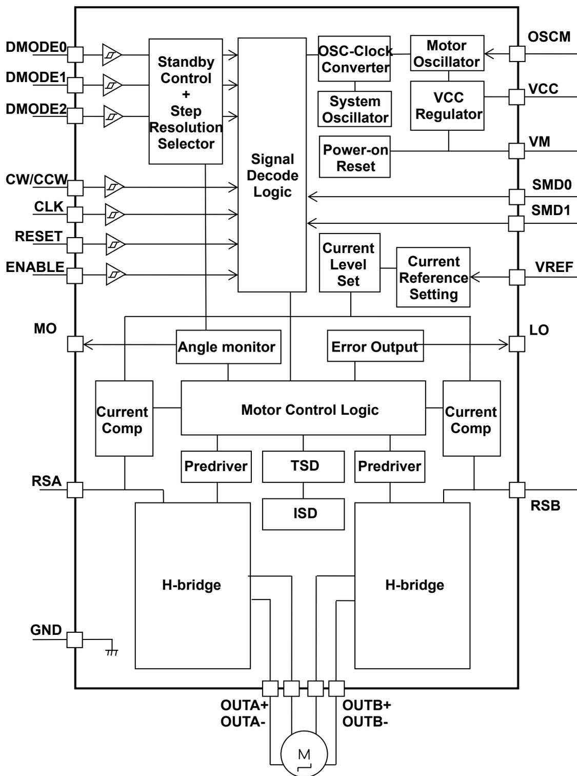
**Figure 3.1 Block Diagram**
