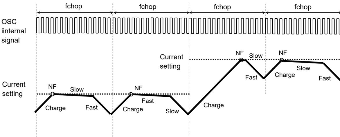
**Figure 6.14 When the next current step is higher**
