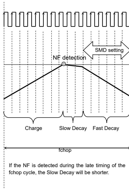
**Figure 6.12 Constant current PWM function and timings (2)**
