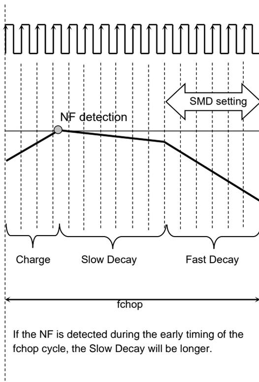
**Figure 6.11 Constant current PWM function and timings (1)**
