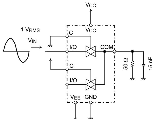
**Figure 6 Cross Talk (between any two switches)**
