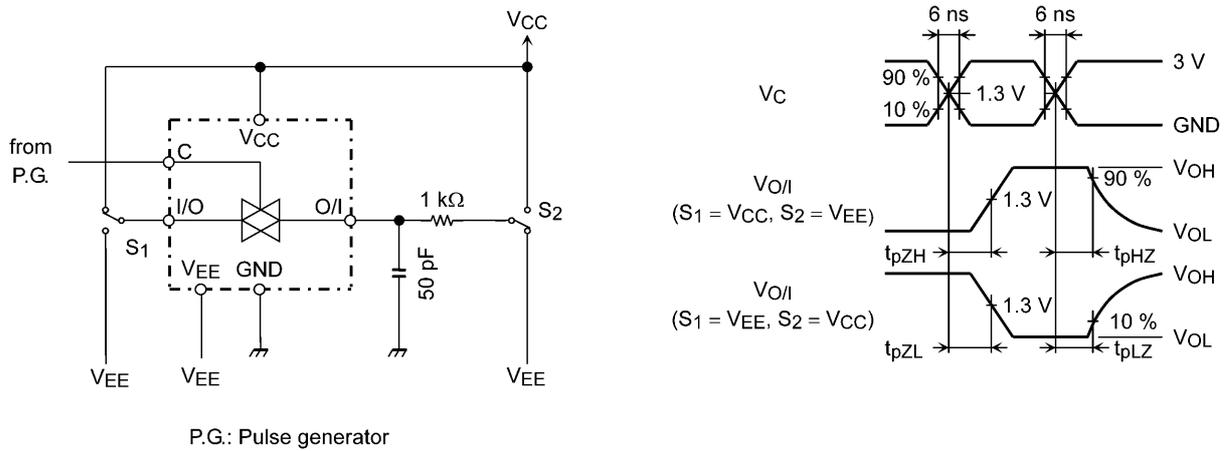
Figure 1  $t_{pLZ}$ ,  $t_{pHZ}$ ,  $t_{pZL}$ ,  $t_{pZH}$
