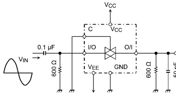
**Figure 4 Feedthrough Attenuation**
