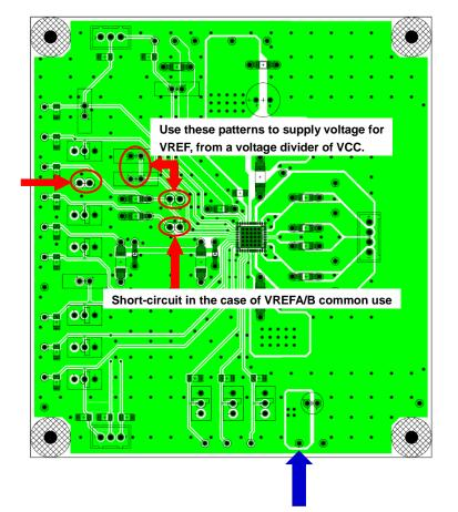
Short the jumper to use the VCC as a power source for the switches.
