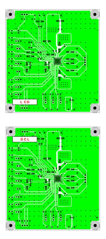
The above figure shows connector positions of D (serial data), C (serial clock), and L (serial latch). When three-line serial output of IC1 is used as three-line serial input of IC2, please connect D, C, and L correctly respectively.
