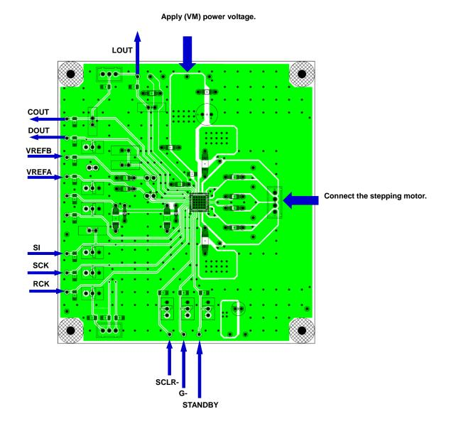
Input each power supply and control signals according to the figure shown above.
