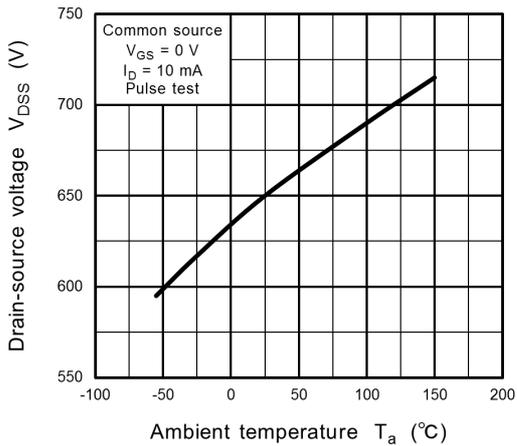
**Fig. 8.5  $V_{DSS} - T_a$**
