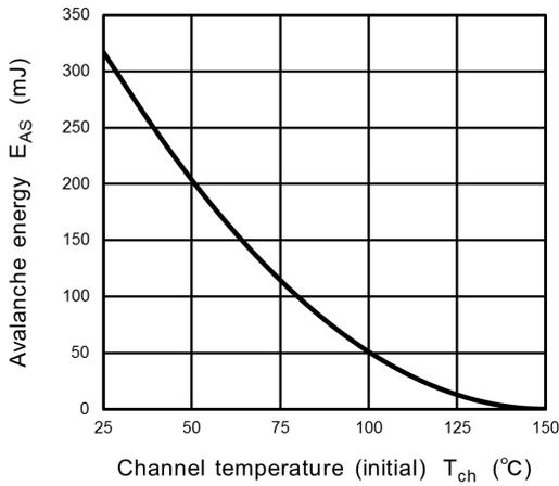
**Fig. 8.14  $E_{AS} - T_{ch}$**
