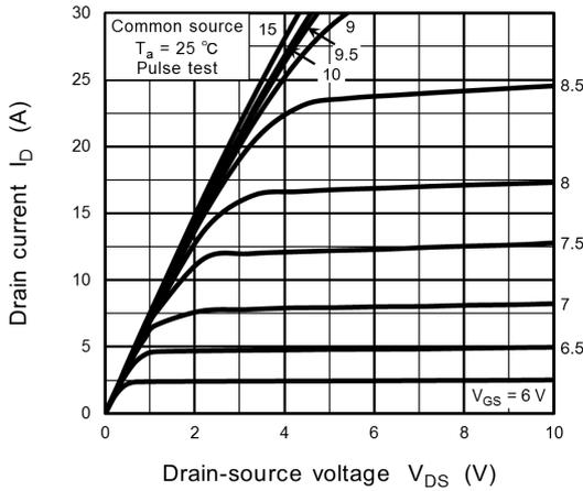
**Fig. 8.1  $I_D - V_{DS}$**
