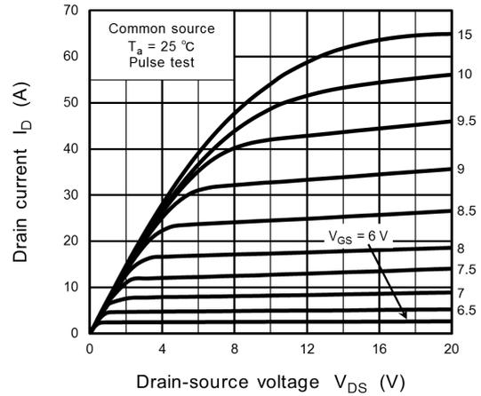
**Fig. 8.2  $I_D - V_{DS}$**
