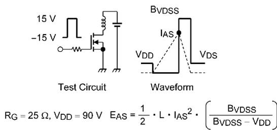
**Fig. 8.16 Test Circuit/Waveform**
