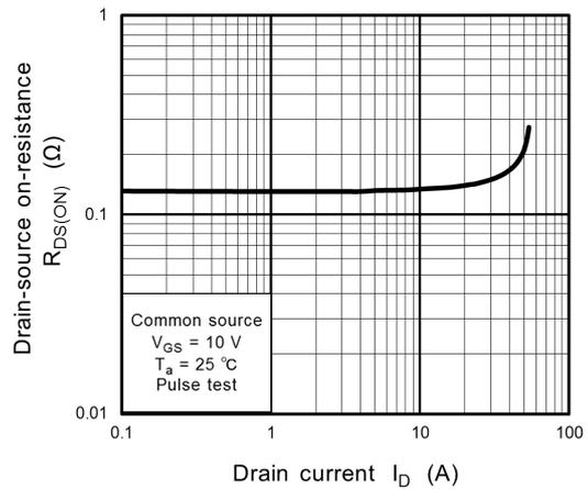
**Fig. 8.6  $R_{DS(ON)} - I_D$**
