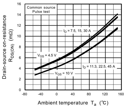
**Fig. 8.9**  $R_{DS(ON)} - T_a$
