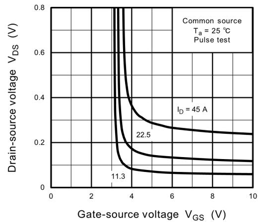
**Fig. 8.4  $V_{DS} - V_{GS}$**
