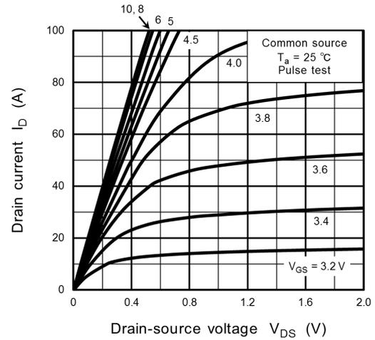
**Fig. 8.2  $I_D - V_{DS}$**
