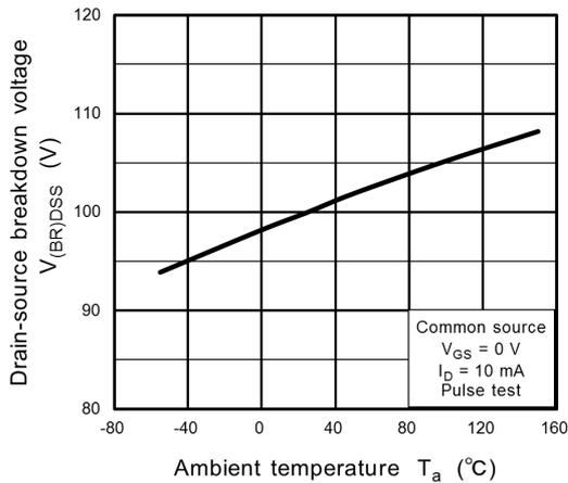
**Fig. 8.7**  $V_{(BR)DSS} - T_a$
