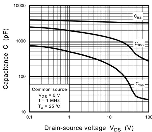
**Fig. 8.11** Capacitance -  $V_{DS}$
