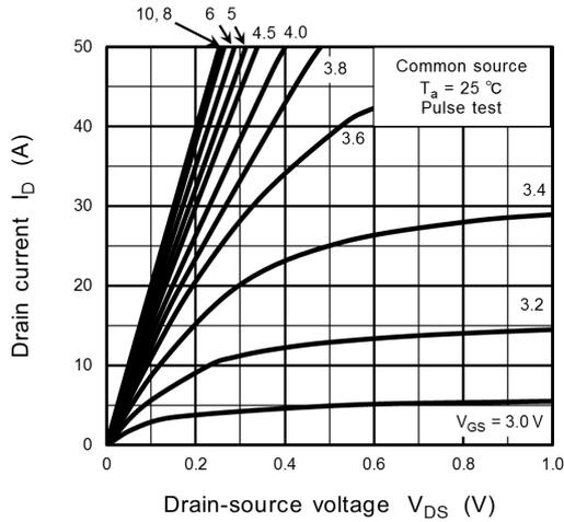
**Fig. 8.1  $I_D - V_{DS}$**
