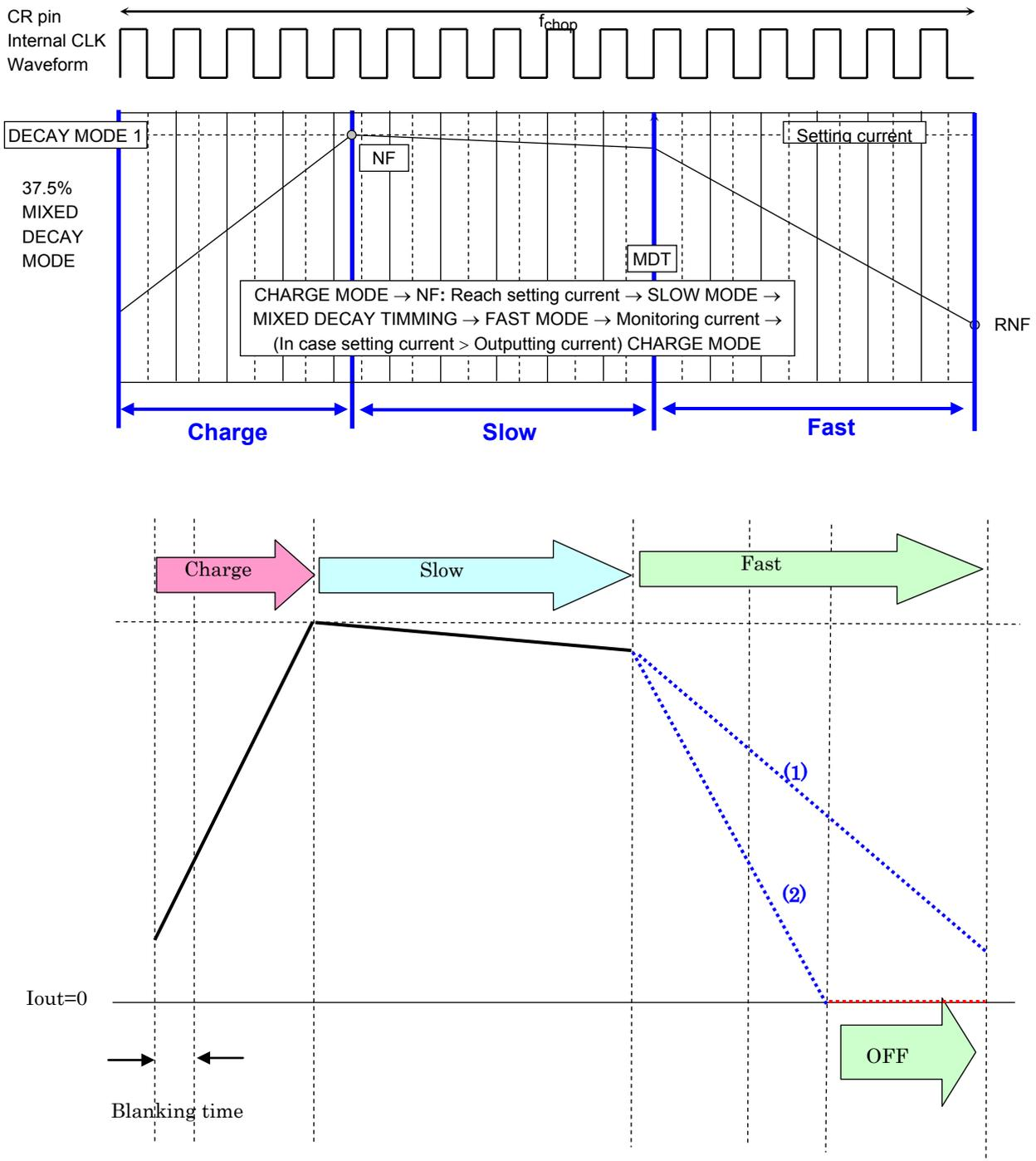
The [NF] shows the point where the output current reaches the setting current value. The [Charge] shows the different value depending on the step resolution characteristics (inductance or resistance).
