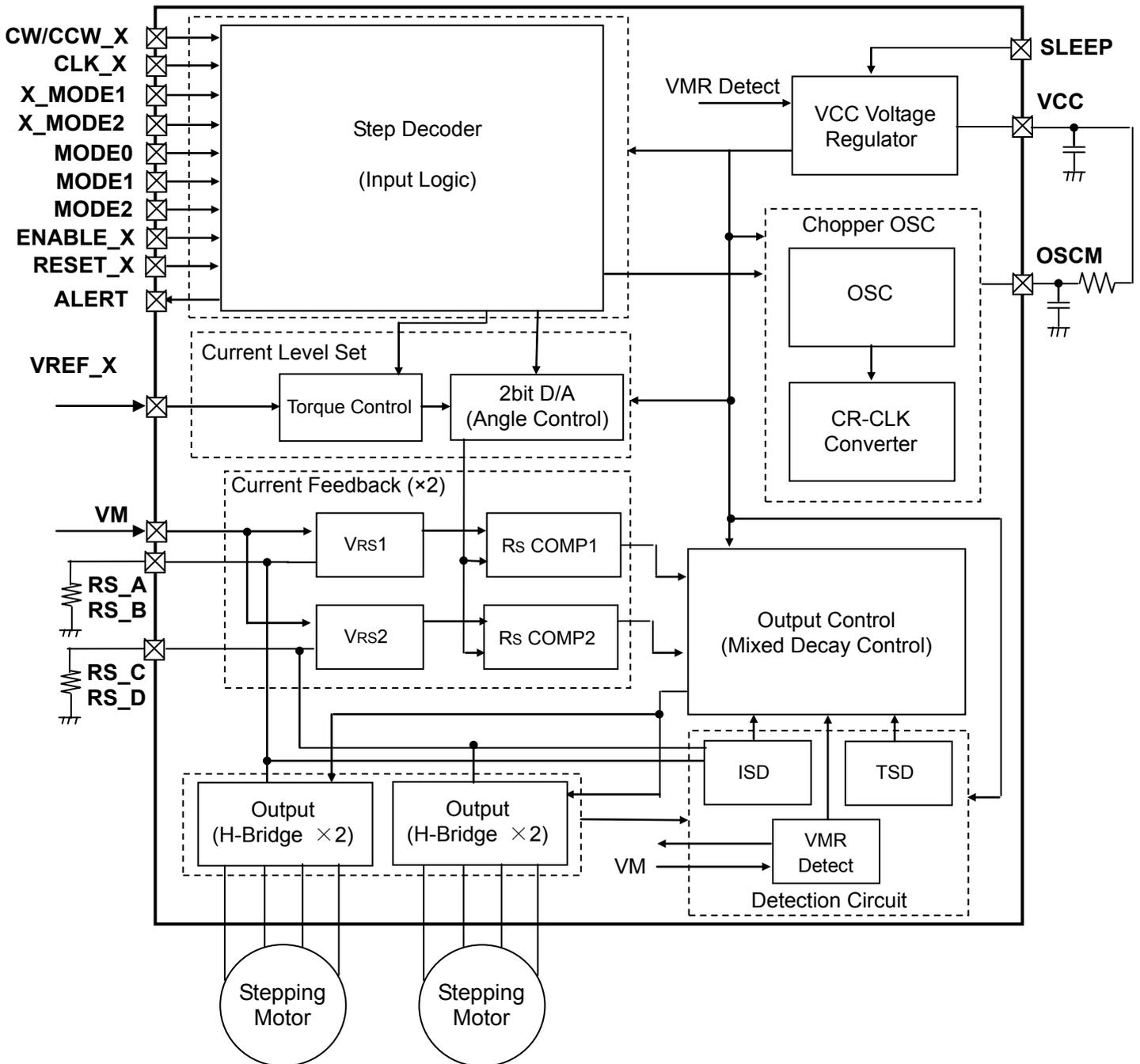
\* "X" means the ellipsis of AB / CD of each Ch. (CW/CCW\_X, CLK\_X, X\_MODE1, X\_MODE2, ENABLE\_X, and RESET\_X)
