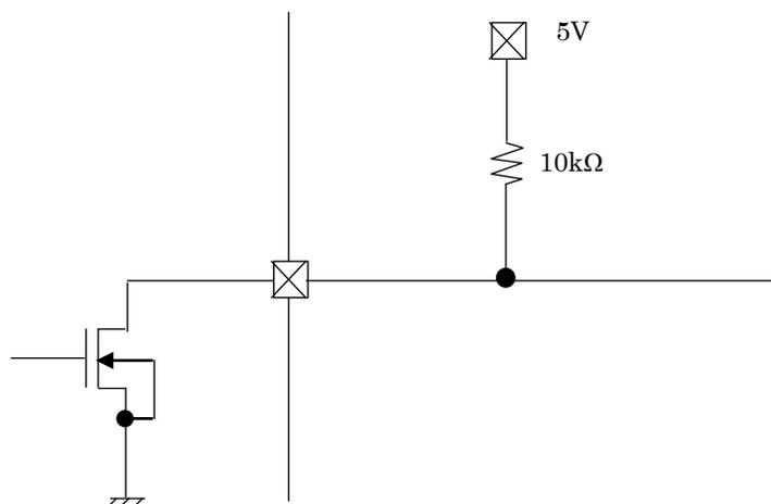
The ALERT is an open drain output pin. When the output pin is pulled up to the VCC with resistance, the low level is output (MOSFET ON) at the Reset, and the high level (internal Hi-Z) is output at the non-reset. Please connect it to the VCC.
