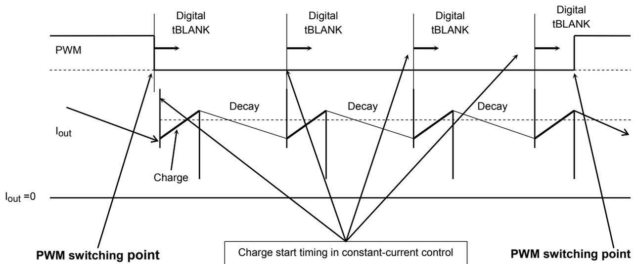
The digital tBLANK time is inserted immediately after the switching timing of externally applied PWM signals,  $CLK\_X$ ,  $ENABLE\_X$  (such as the switching timing between short brake and charging), and also when the charging in constant-current chopper drive is started.
