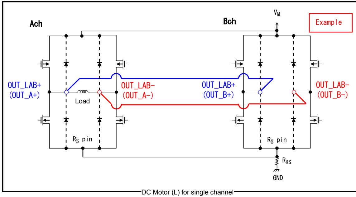
○ ...Indicates an IC output pin connected to a motor.
