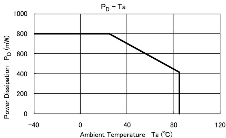
Please allow sufficient margin when designing a board pattern to fit the expected power dissipation. Also take into consideration the ambient temperature, input voltage, output current, etc. and applying the appropriate derating for allowable power dissipation during operation.
