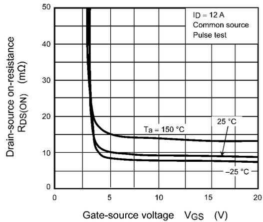
**Fig. 9.4  $R_{DS(ON)} - V_{GS}$**
