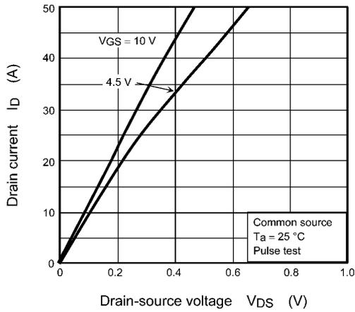
**Fig. 9.1  $I_D - V_{DS}$**
