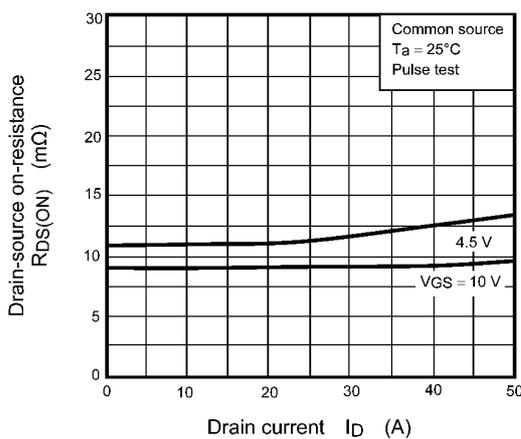
**Fig. 9.5  $R_{DS(ON)} - I_D$**
