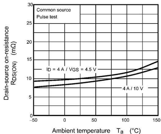
**Fig. 9.6  $R_{DS(ON)} - T_a$**
