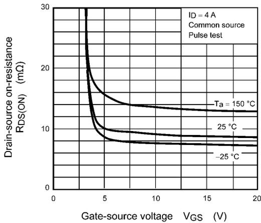
**Fig. 9.3  $R_{DS(ON)} - V_{GS}$**
