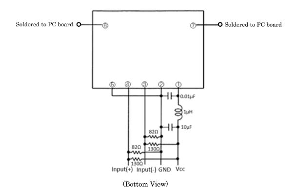
Note.7 : Place termination resistors near physical layer device data input pin. Make differential signal paths short and the same length. Use ground plane(or multi-layer)printed circuit board for best high frequency performance. Signal trace should be 50  $\Omega$  transmission lines(micro strip or strip line). Use high-frequency monolithic ceramic bypass capacitors and low DC resistance inductors.
