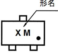
A schematic diagram of a rectangular component, identical in shape to the one above. The letters "X M" are printed in the center, and a small black dot is located on the right side. A leader line points from the text "形名" (Form Name) above to the top edge of the component.                        |
