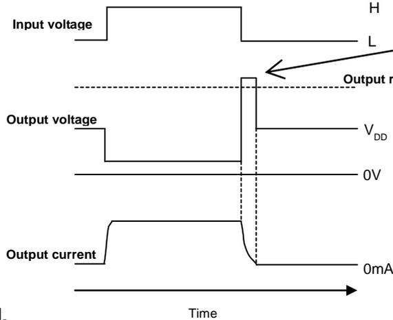
In switching from ON to OFF, the inductive load may generate high voltage which exceeds output rating under the influence of back electromotive force.
