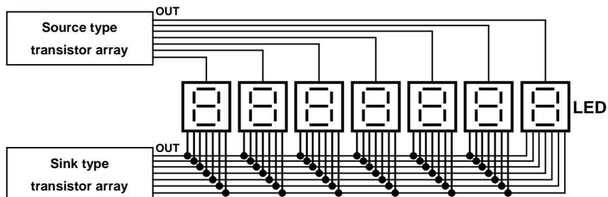
**Construction of output circuit**
