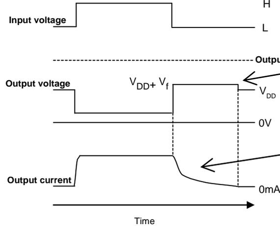
Generation of back electromotive force which exceeds output rating is avoided by discharging through the clamp diode in the IC.
