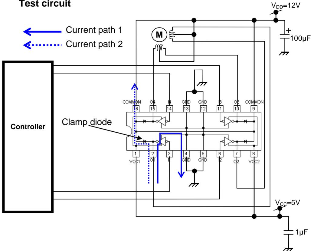
When clamp diode and zener diode are used.
