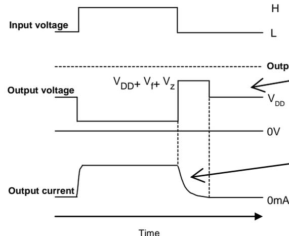
Problem of degrading time of falling current in switching off is solved by connecting the zener to COMMON pin.
