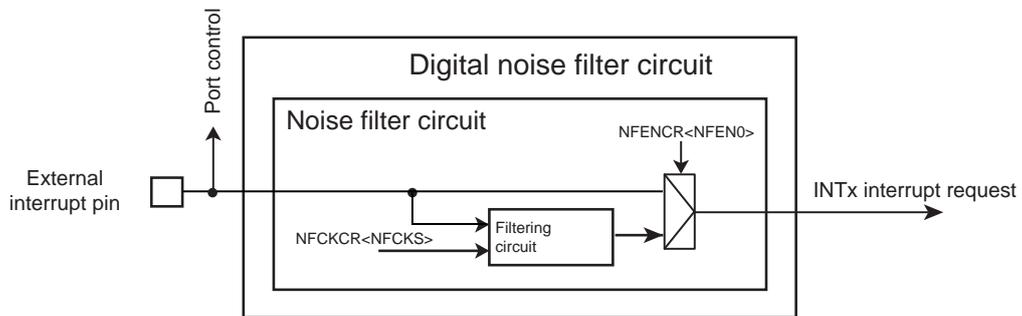
Figure 9-1 Circuit diagram of digital noise filter
