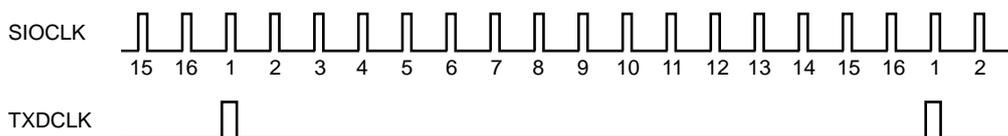
Figure 13-7 Generation of Transmission Clock in UART mode
