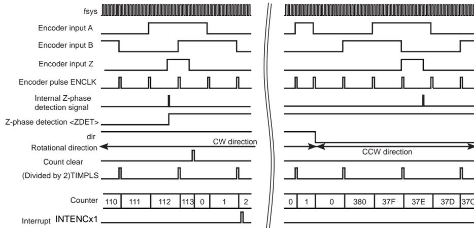
In encoder mode, the incremental encoder inputs should be connected to the ENCA, ENCB, and ENCZ pins. The encoder multiplies the ENCA and the ENCB signals into 4 to count the encoder pulses.
