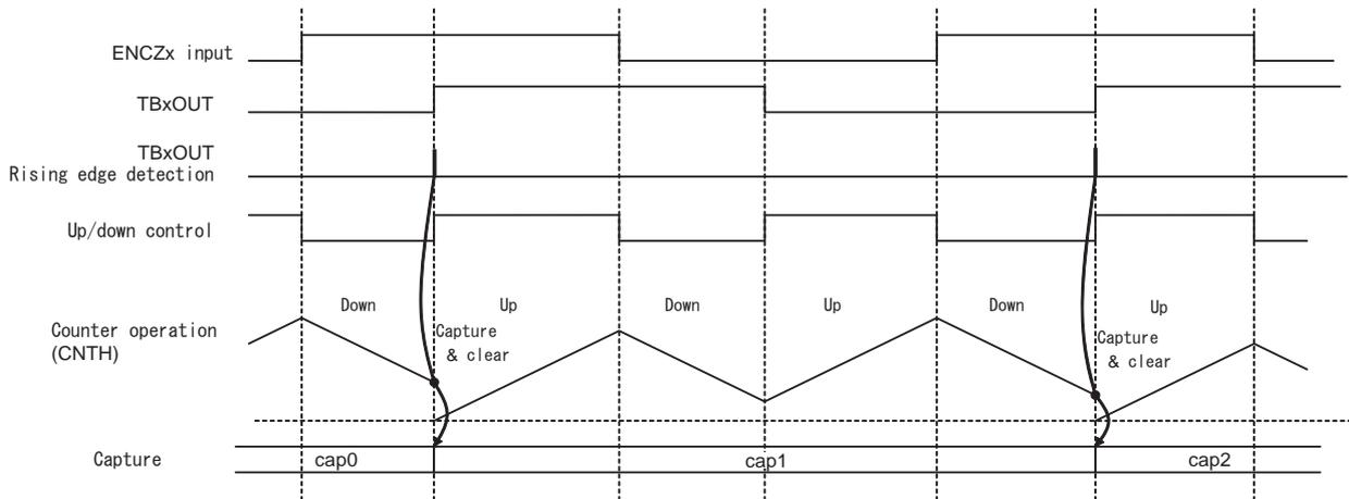
Figure 19-2 Operation in phase counter mode (phase difference)
