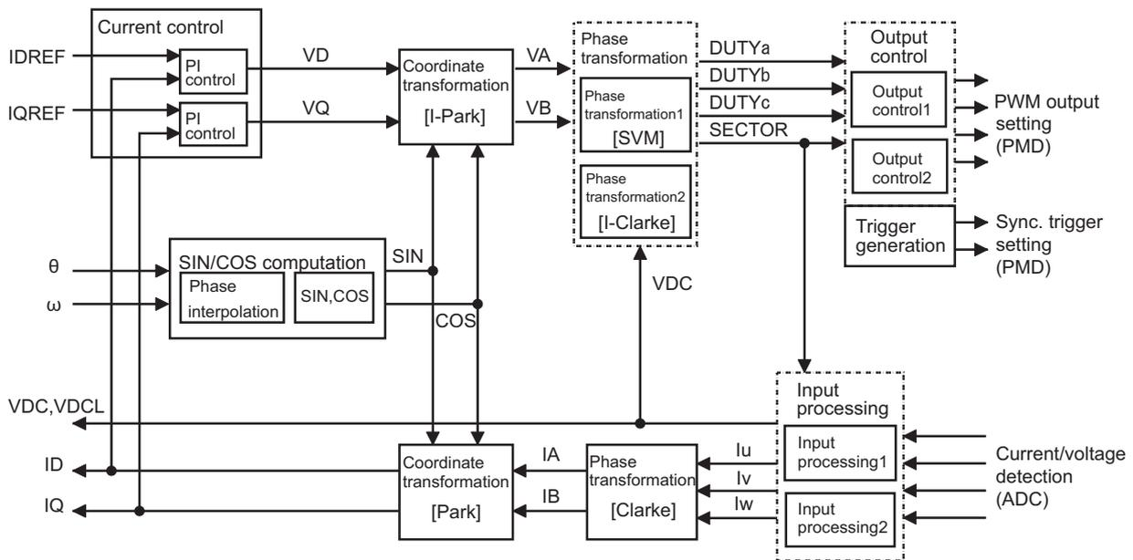
Figure 18-1 Block diagram of the vector control circuit
