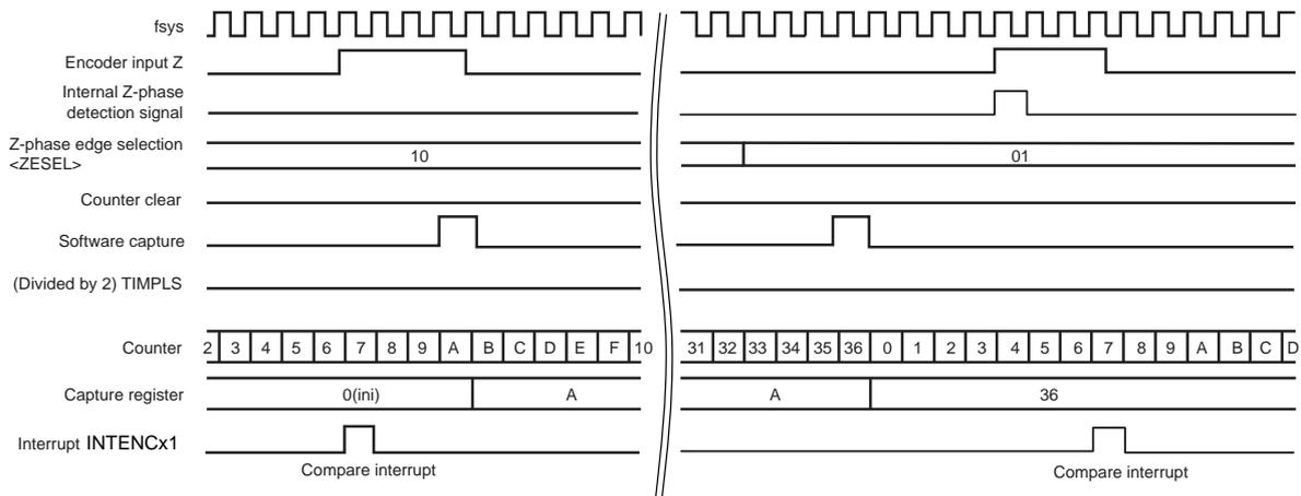
When <ZEN> = "1", a Z-input can work as the external trigger. When <ZEN> = "0", the external trigger is not used.
