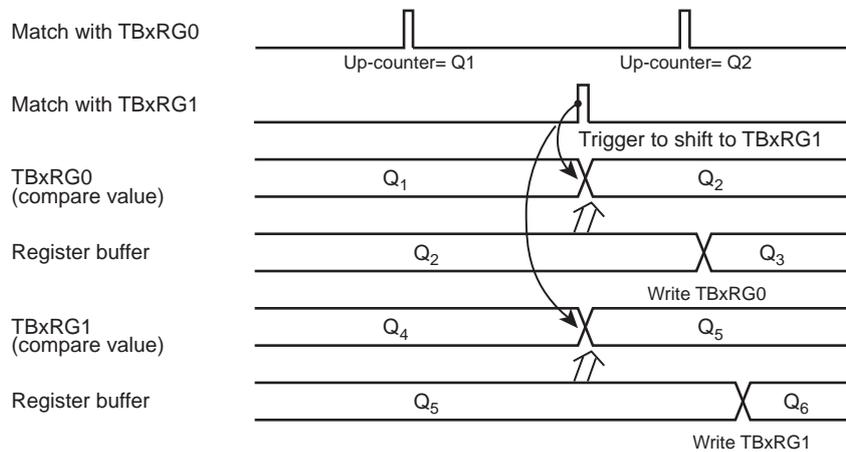
Figure 12-3 Register Buffer Operation
