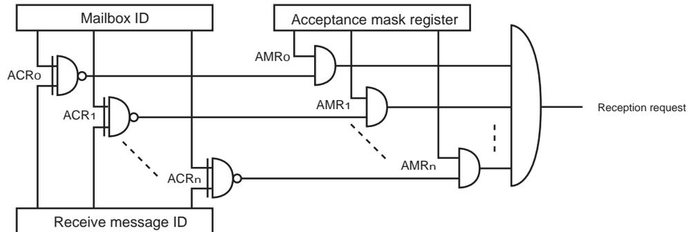
Figure 15-4 Receive filtering
