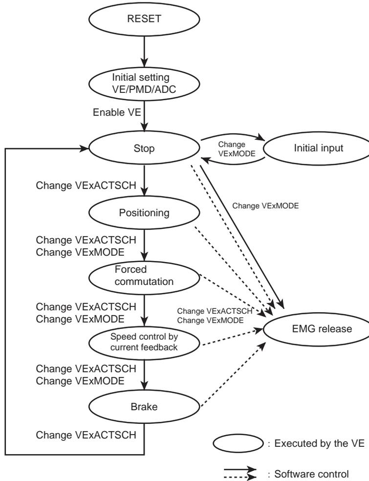
Figure 18-8 Example of Motor Control Operation Status Flowchart
