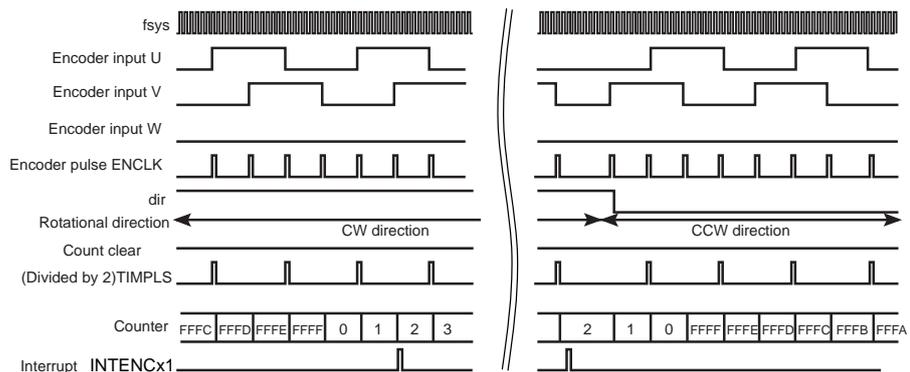
Hall sensor inputs (U,V, and W) should be connected to ENCAx, ENCBx, and ENCZx. When <P3EN> = "0", the counter multiplies a 2-phase input (ENCAx or ENCBx) by 4; when <P3EN> = "1", the counter multiplies a 3-phase input (ENCAx, ENCBx, or ENCZx) by 6. After that, the counter counts the Hall sensor pulse.
