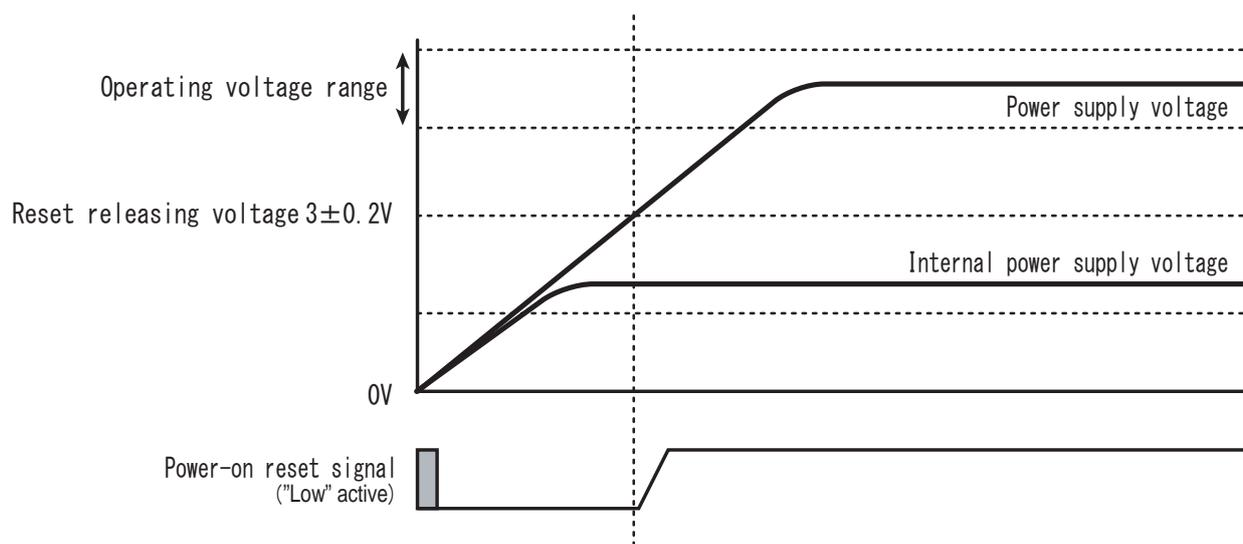
Figure 20-2 Power-on-reset operation timing at power-on
