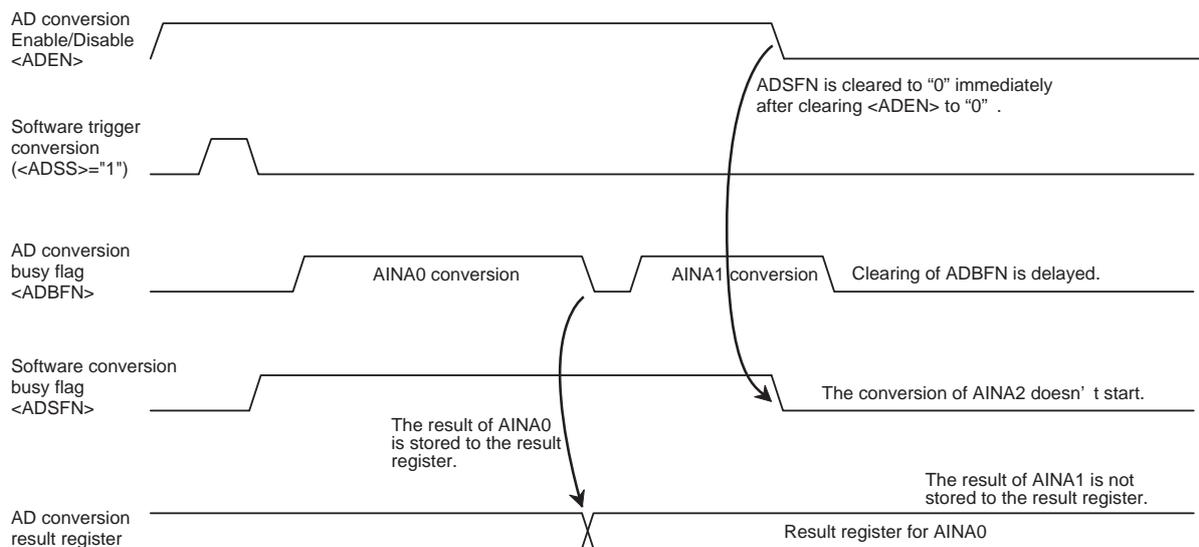
Figure 16-5 Writing "0" to <ADEN> during the software trigger AD conversion
