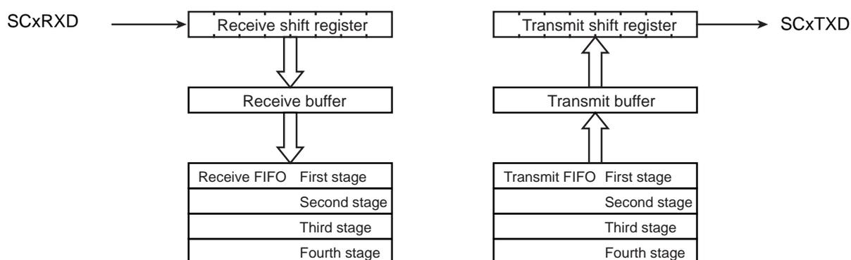
Figure 13-4 The Configuration of Buffer and FIFO
