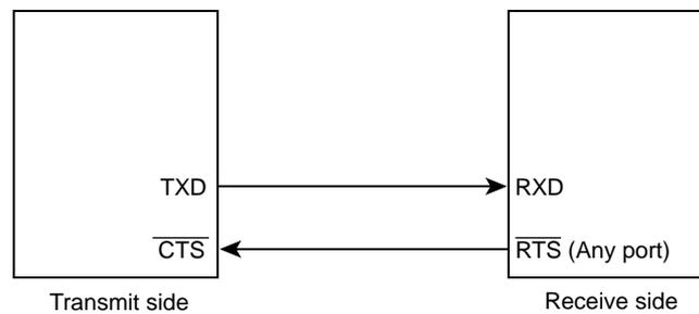
Figure 13-11 Handshake Function
