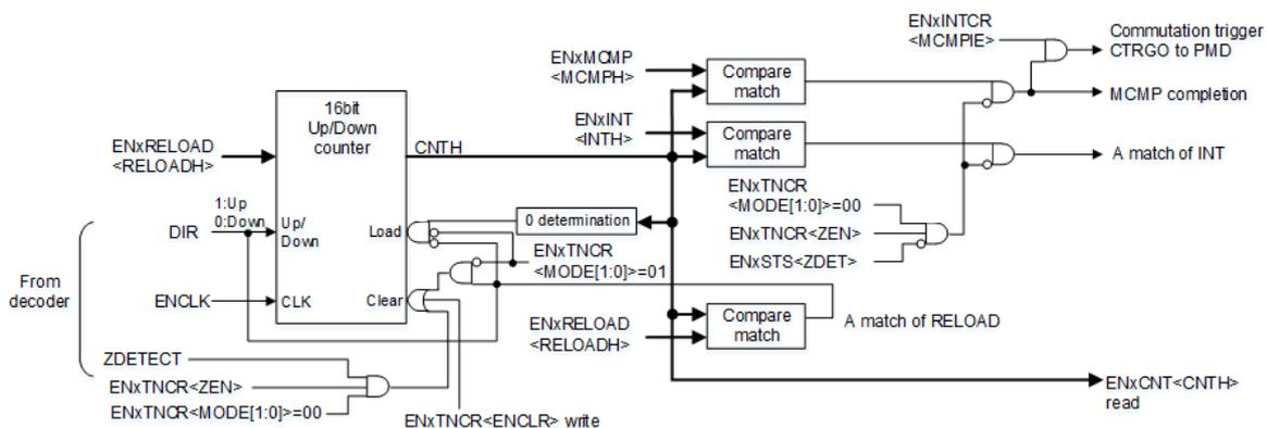
Figure 19-11 Configuration of the counter (encoder mode and sensor mode (event count))
