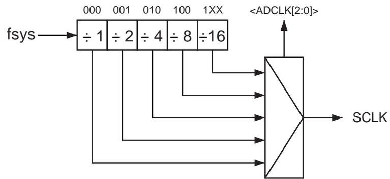
Note 1: Frequency of SCLK can be used up to 120MHz.
