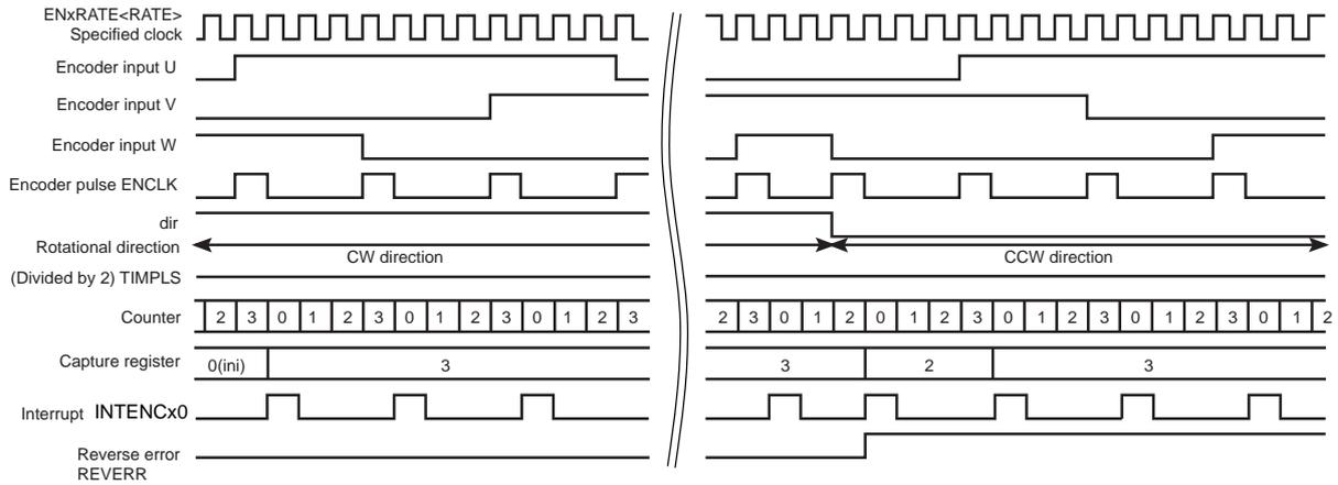
2. 2-phase decoding (ENxTNCR<P3EN> = 0)
