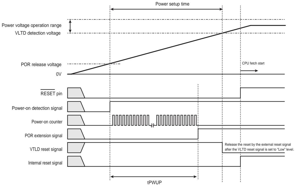
Figure 5-4 Reset Operation by  $\overline{\text{RESET}}$  pin (Reset operation by VLTD is valid.)
