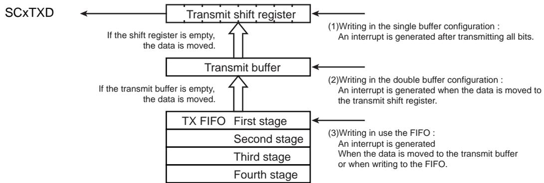
Figure 13-14 Transmit Buffer / FIFO Configuration Diagram
