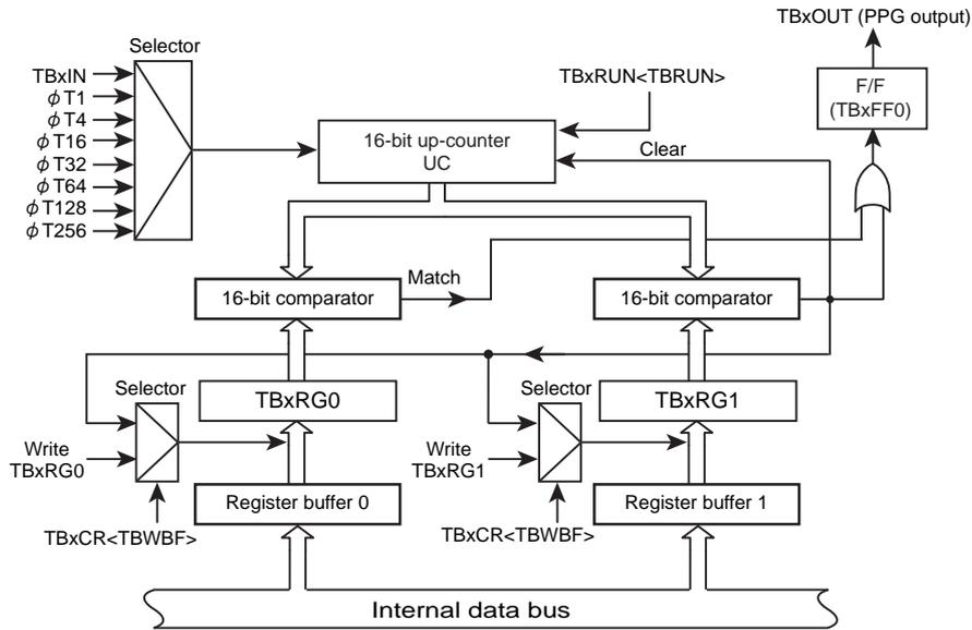
Figure 12-4 Block Diagram of 16-bit PPG Mode
