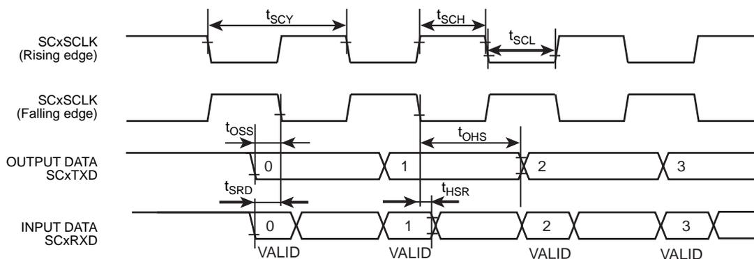
Figure 27-1 Serial channel timing(SIO)
