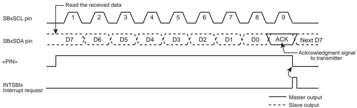
Figure 14-8 <BC[2:0]>= "000", <ACK>= "1" (Receiver Mode)
