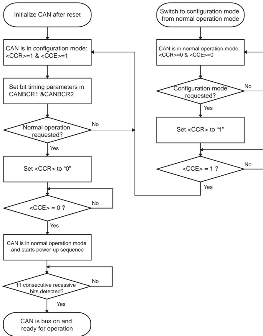
Figure 15-7 Flowchart of Initial Setup of CAN Controller
