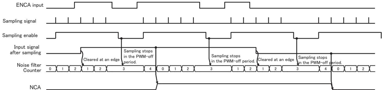
Figure 19-6 Noise cancelling (Sampling in the PWM-on period. Noise cancelling timer stops in the PWM-off period. <NCT>=4)
