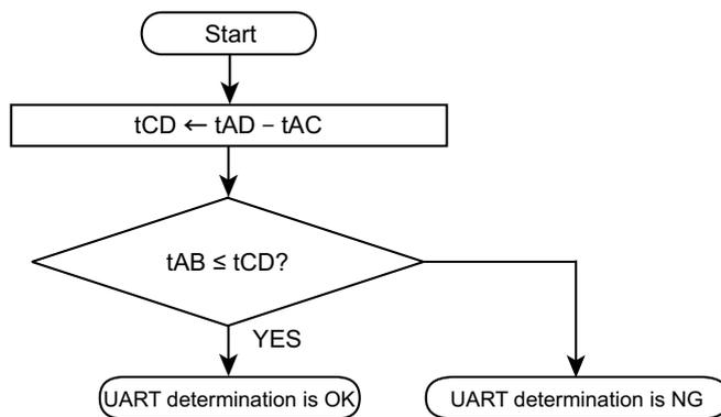
Figure 24-9 Serial operation mode determination flow chart
