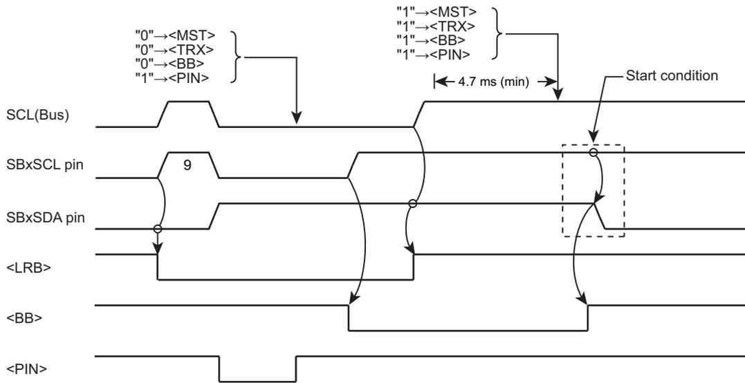
Figure 14-11 Timing Chart of Generating a Restart
