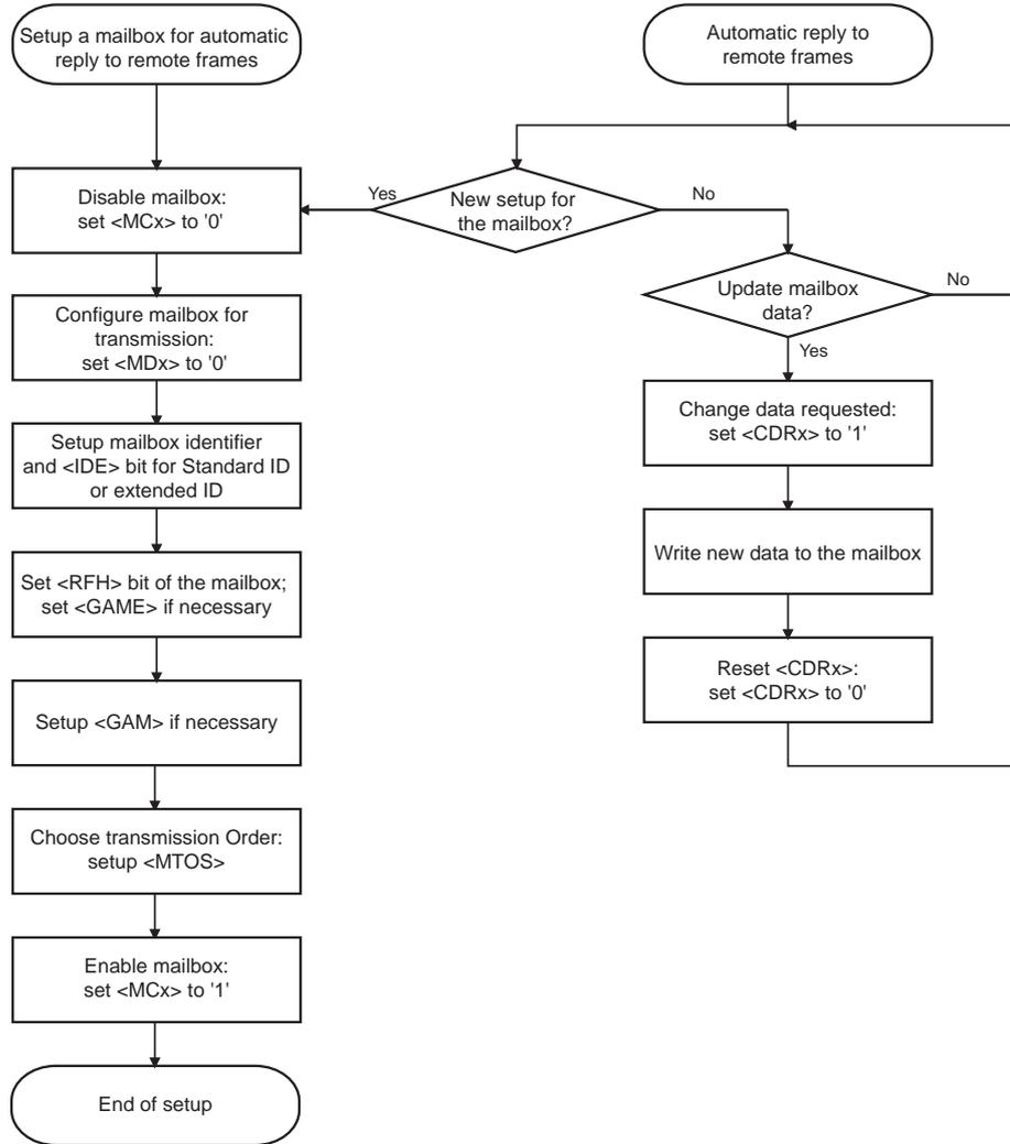
Figure 15-11 Flowchart of Remote Frame Handling Using the Automatic Reply Feature
