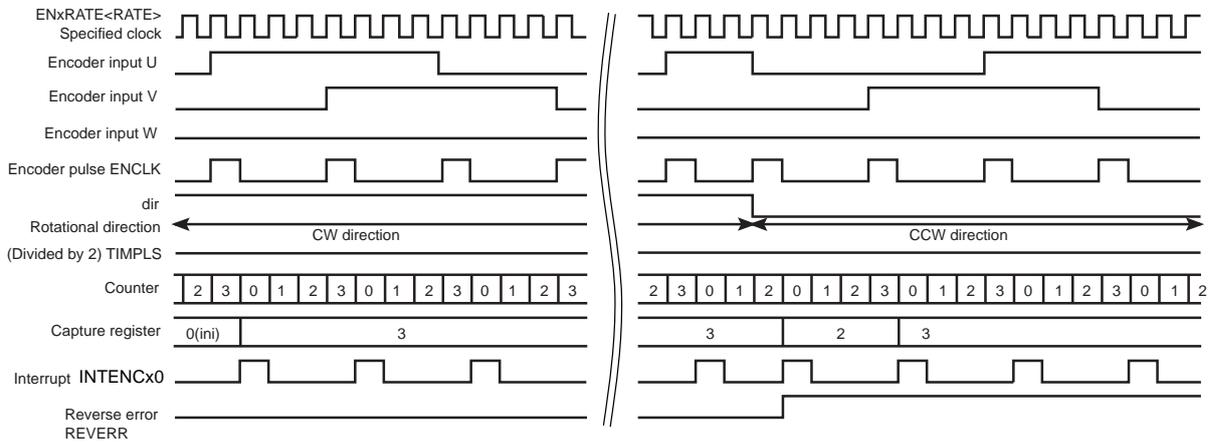
Hall sensor inputs (U, V, and W) should be connected to ENCAx, ENCBx, and ENCZx. When <P3EN> = "0", the counter multiplies a 2-phase input (ENCAx or ENCBx) by 4; when <P3EN> = "1", the counter multiplies a 3-phase input (ENCAx, ENCBx, or ENCZx) by 6. After that, the counter generates a 4-fold or 6-fold rotational edge pulse (ENCLK).
