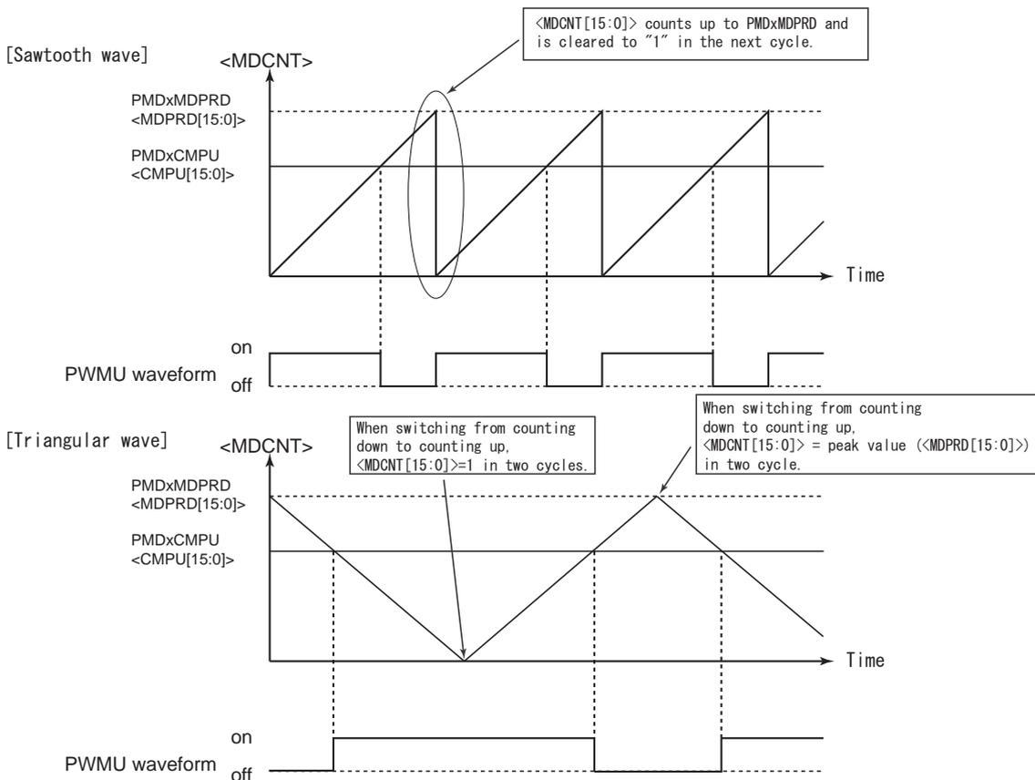
Figure 17-5 PWM Waveforms
