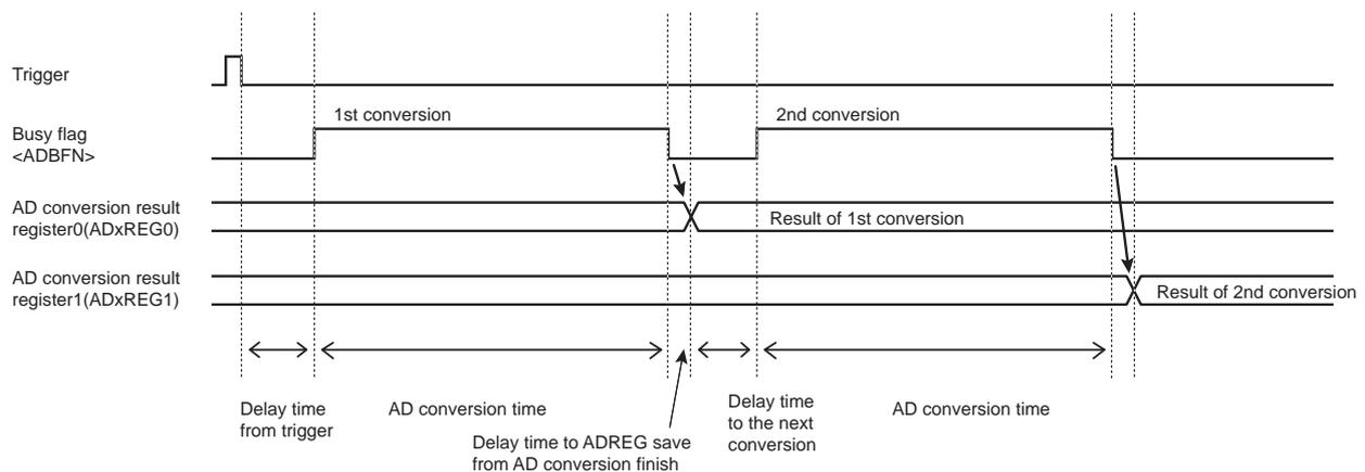
Figure 16-3 Timing chart of AD conversion
