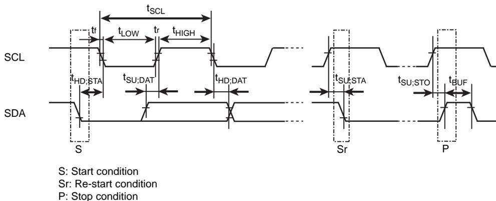
Figure 27-2 Serial bus timing (I2C)
