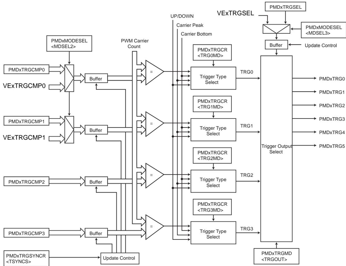
Figure 17-12 Sync Trigger Generation Circuit
