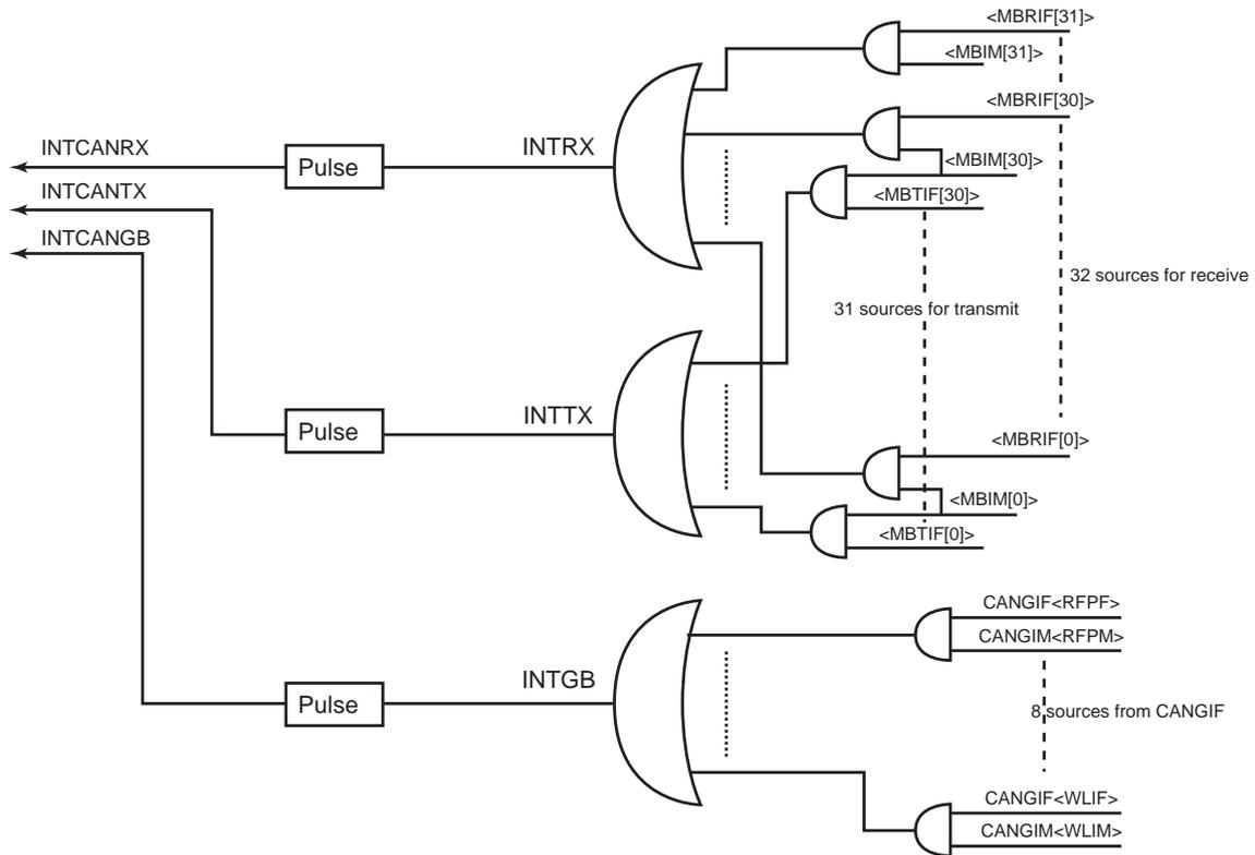
Figure 15-6 Block Diagram of CAN interrupt signals
