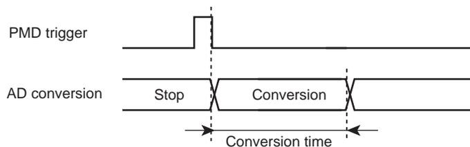
Figure 18-7 ADC conversion time
