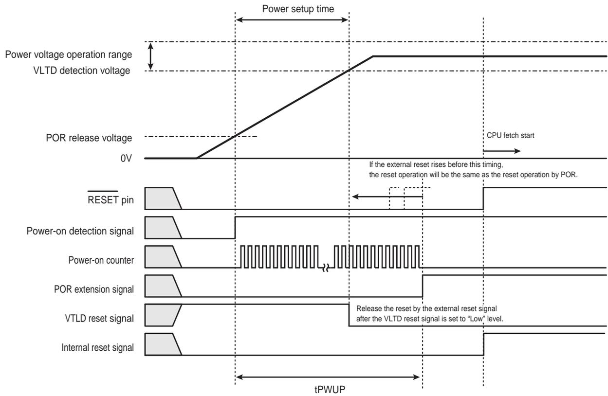
Figure 5-3 Reset Operation by  $\overline{\text{RESET}}$  pin (Reset operation by POR is valid.)
