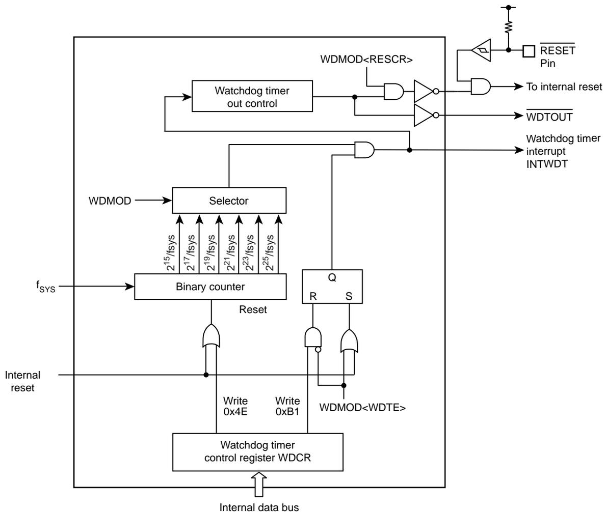
Figure 23-1 Block Diagram of the watchdog Timer
