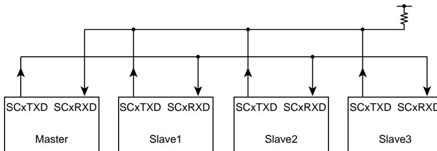
Figure 13-21 Serial Links to Use Wake-up Function
