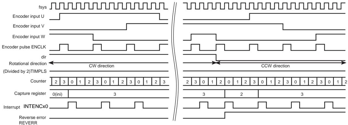
2. 2-phase decoding (ENxTNCR<P3EN> = 0)
