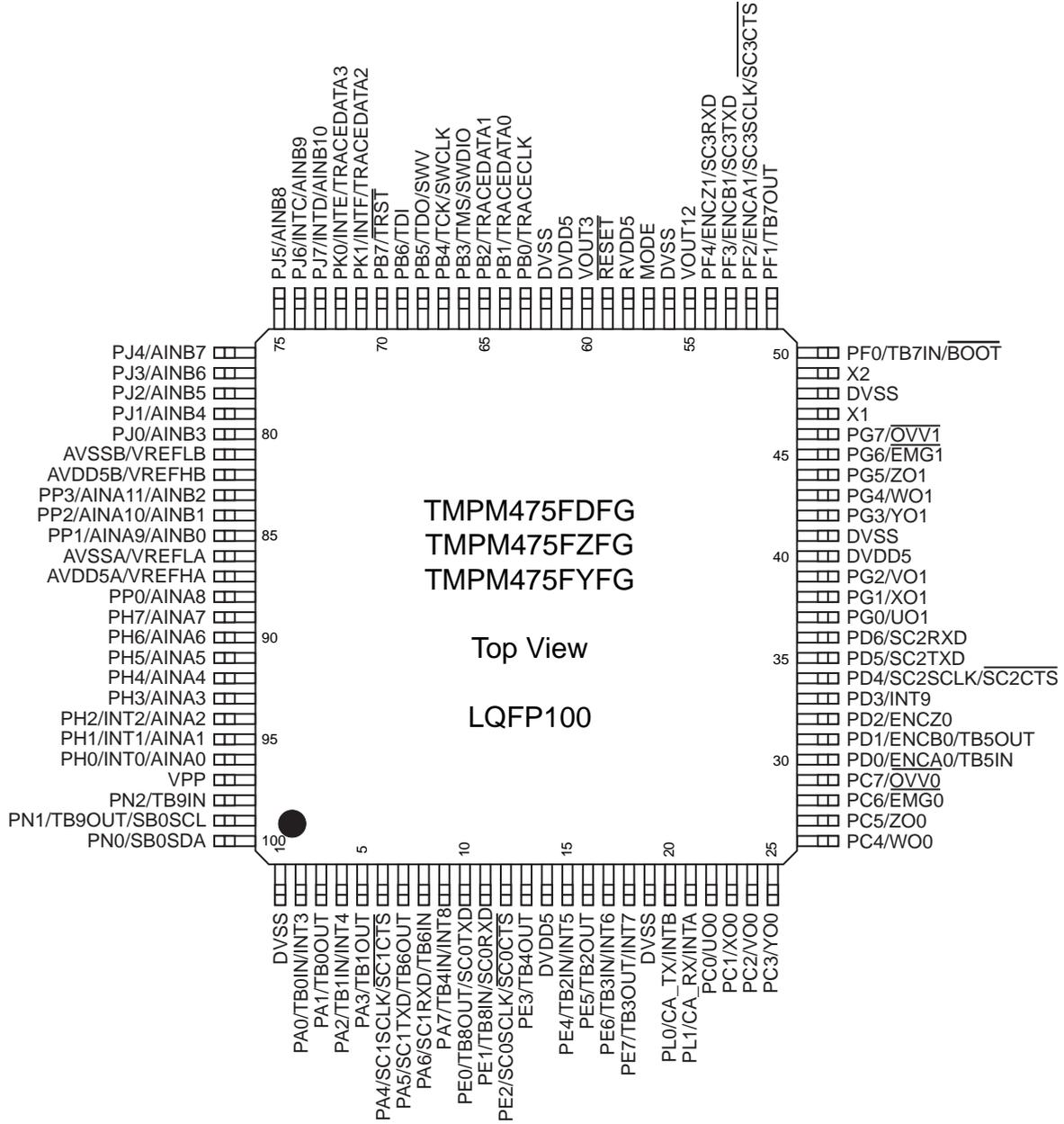
Figure 1-2 Pin layout (LQFP100)
