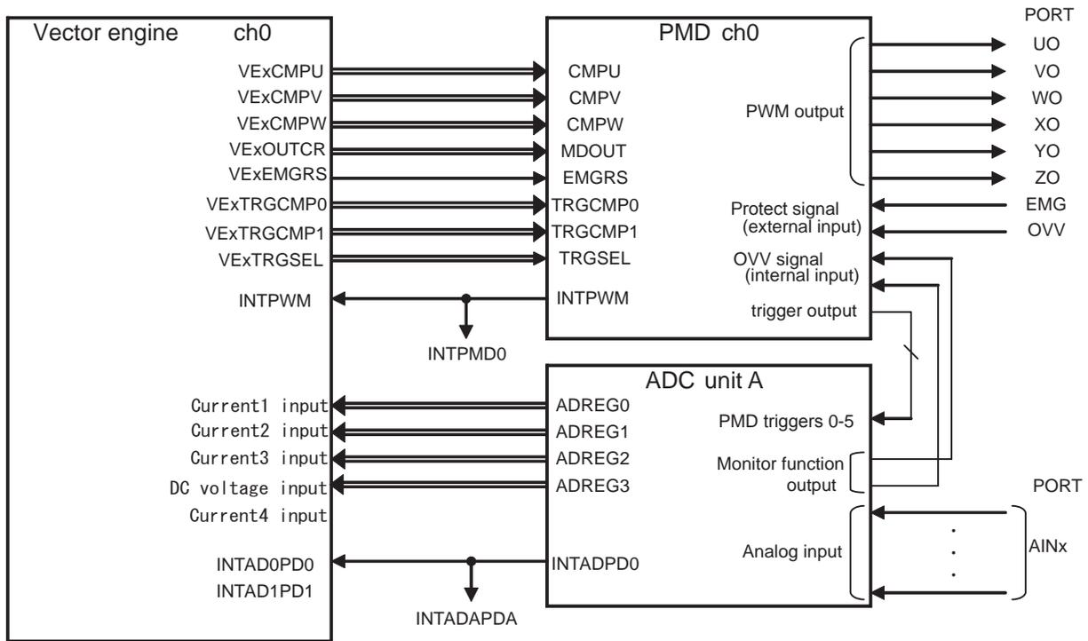
Figure 17-2 Related diagram of Motor control circuit, Vector engine and A/D converter
