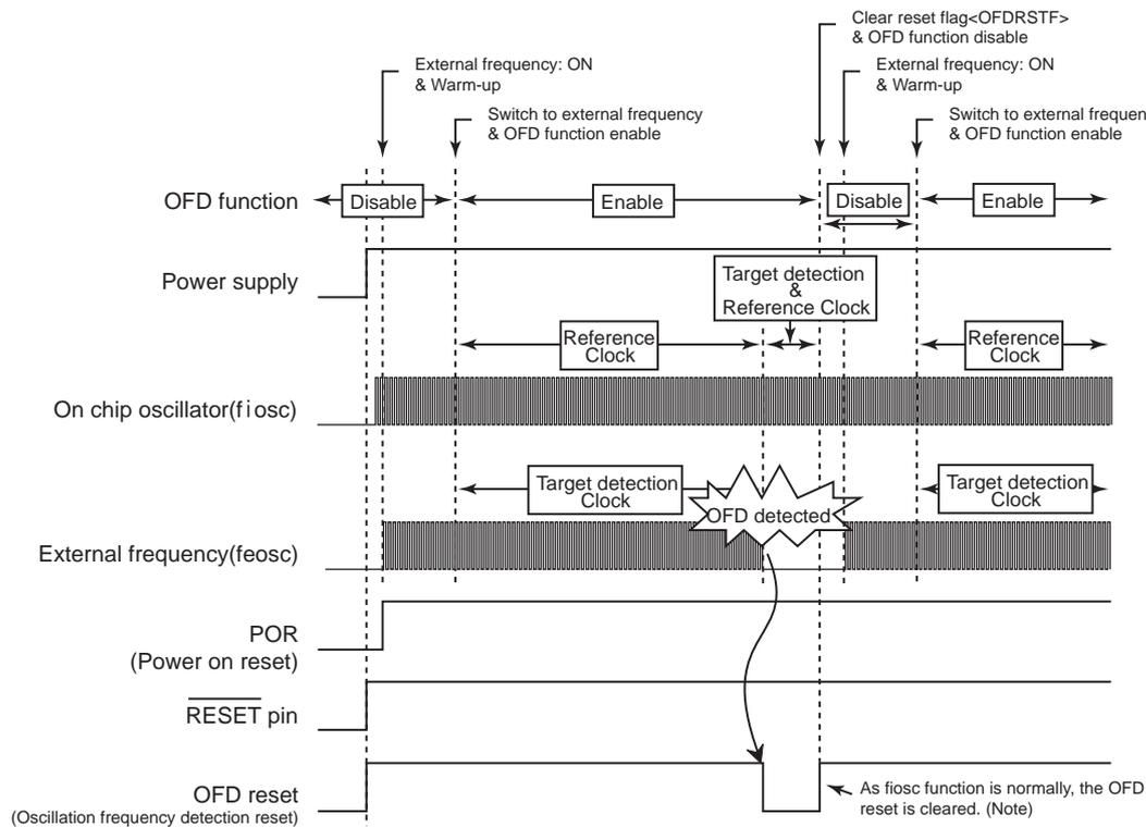
Note: The target clock is set without 10MHz into OFDMNPLLOFF and OFDMXPLLOFF. (eg, setting to 8MHz value to these registers) And when the target clock frequency is  $f_{osc}$  and the reset generated by OFD, the reset might be generated continuously due to as abnormal detection until OFD detects correctly.
