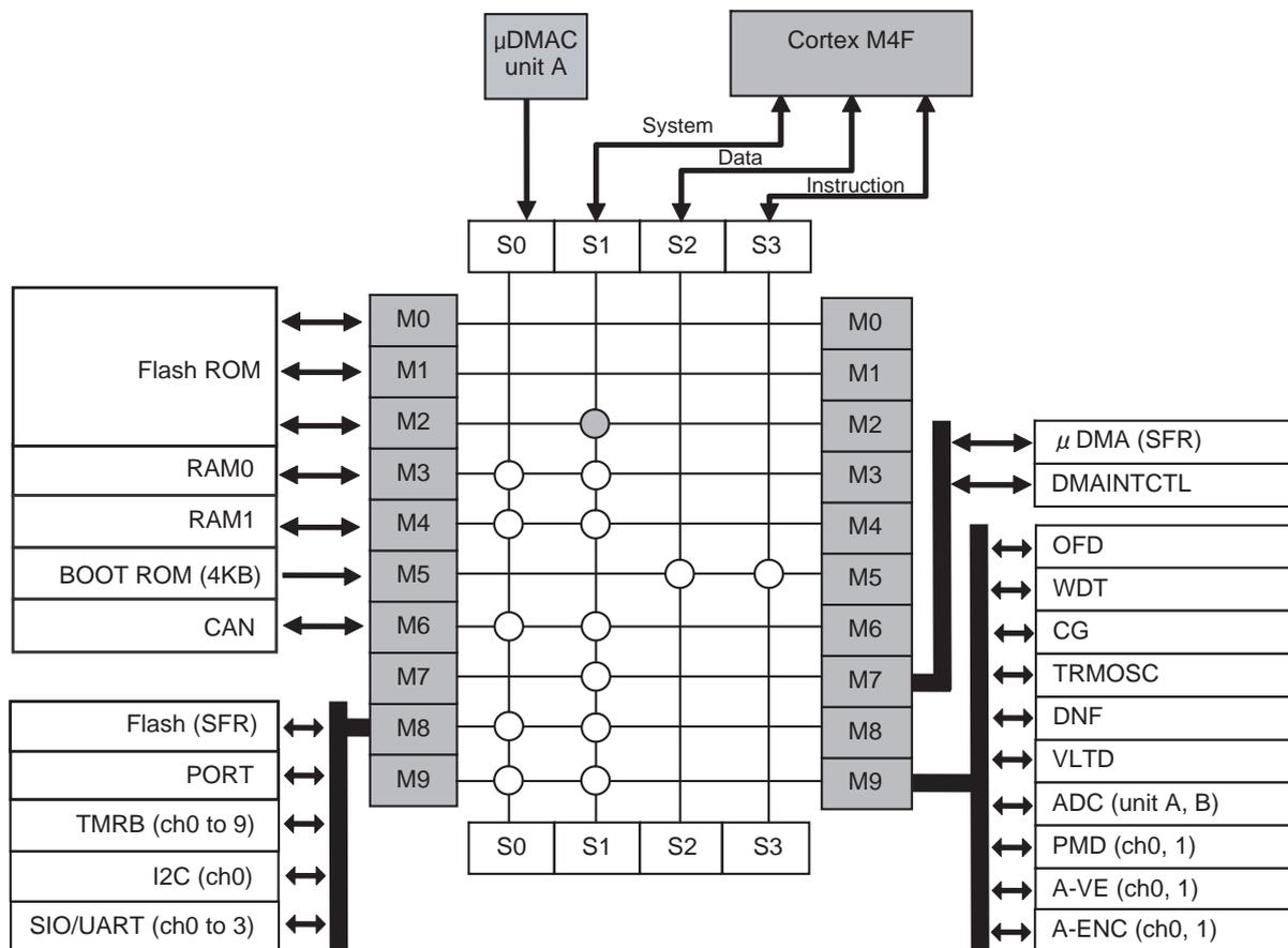
Figure 4-5 Bus Matrix of TMPM475FDFG/FZFG/FYFG
