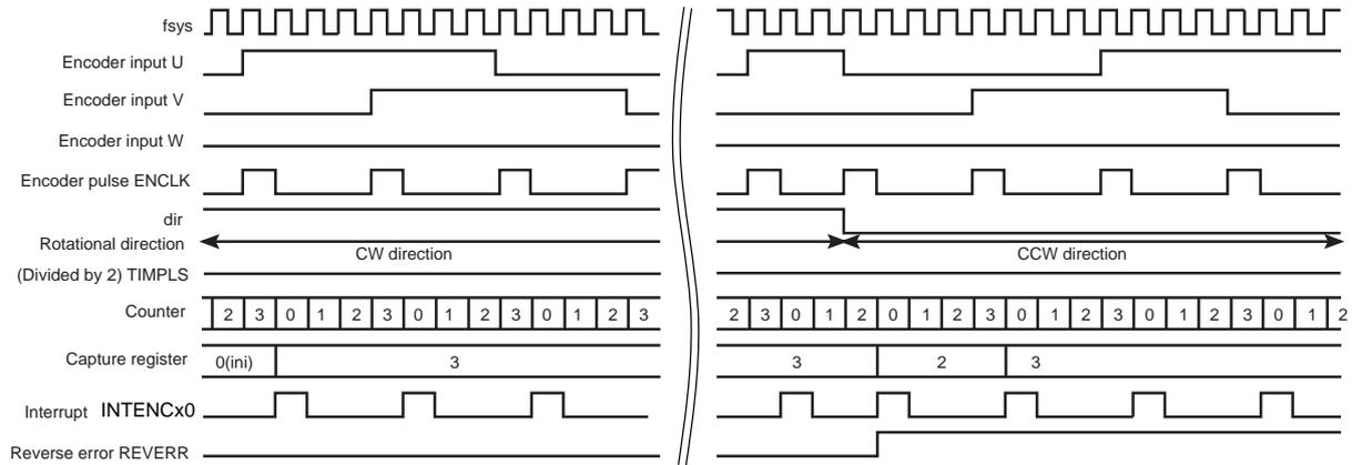
Hall sensor inputs (U, V, and W) should be connected to ENCAx, ENCBx, and ENCZx. When  $\langle P3EN \rangle = "0"$ , the counter multiplies a 2-phase input (ENCAx or ENCBx) by 4; when  $\langle P3EN \rangle = "1"$ , the counter multiplies a 3-phase input (ENCAx, ENCBx, or ENCZx) by 6. After that, the counter generates a 4-fold or 6-fold rotational edge pulse (ENCLK).
