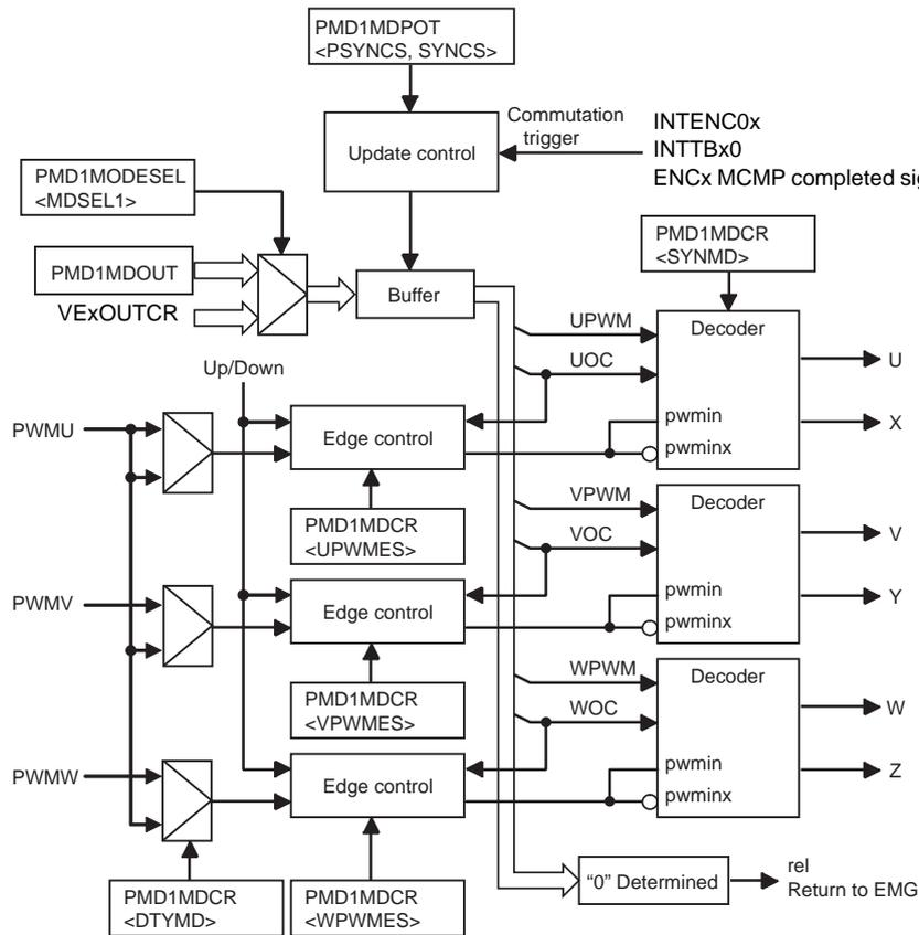
Figure 17-7 Conduction Control Circuit
