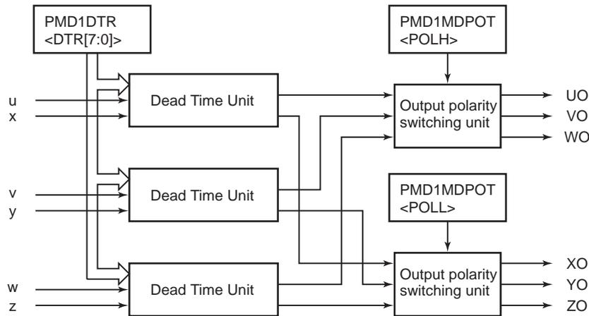
Figure 17-9 Dead Time Control Circuit
