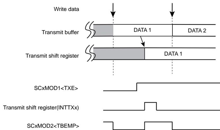
Figure 13-8 Operation of Transmit Buffer (Double-buffer is enabled)
