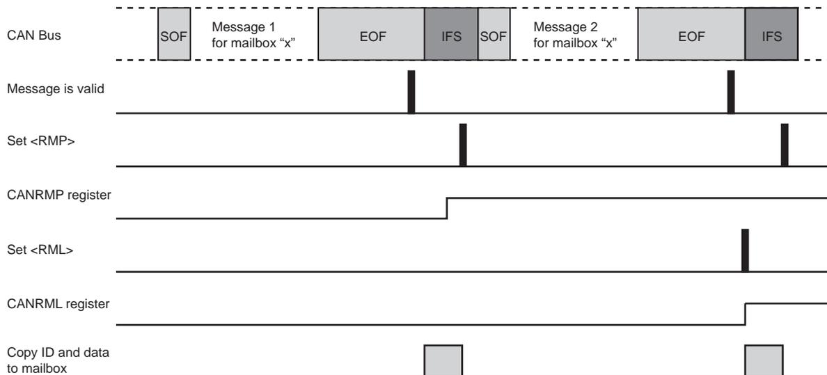
Figure 15-3 Timing when a Receive Message Lost Occurs
