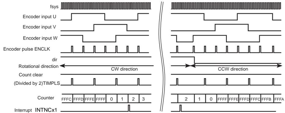
2. 2-phase decoding (ENxTNCR<P3EN> = 0)
