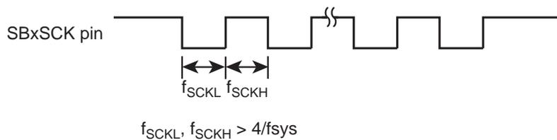
Figure 14-14 Maximum Transfer Frequency of External Clock Input
