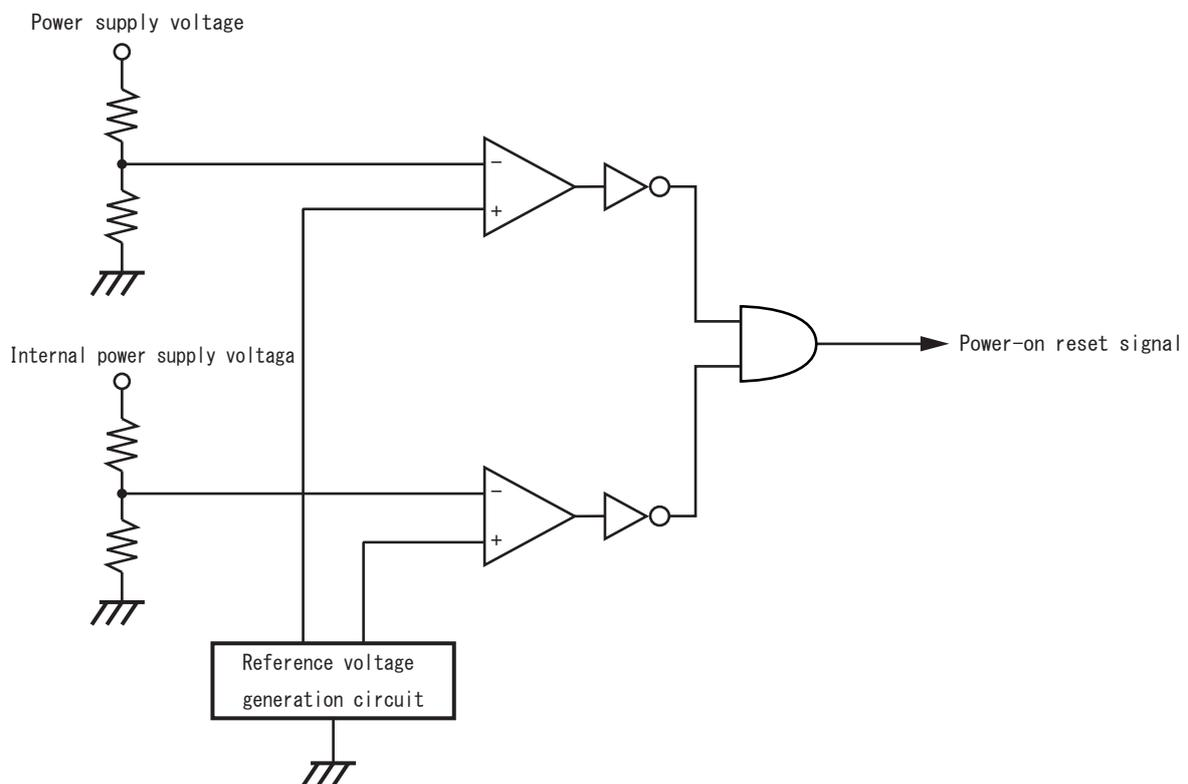
Figure 20-1 Power-on-reset circuit
