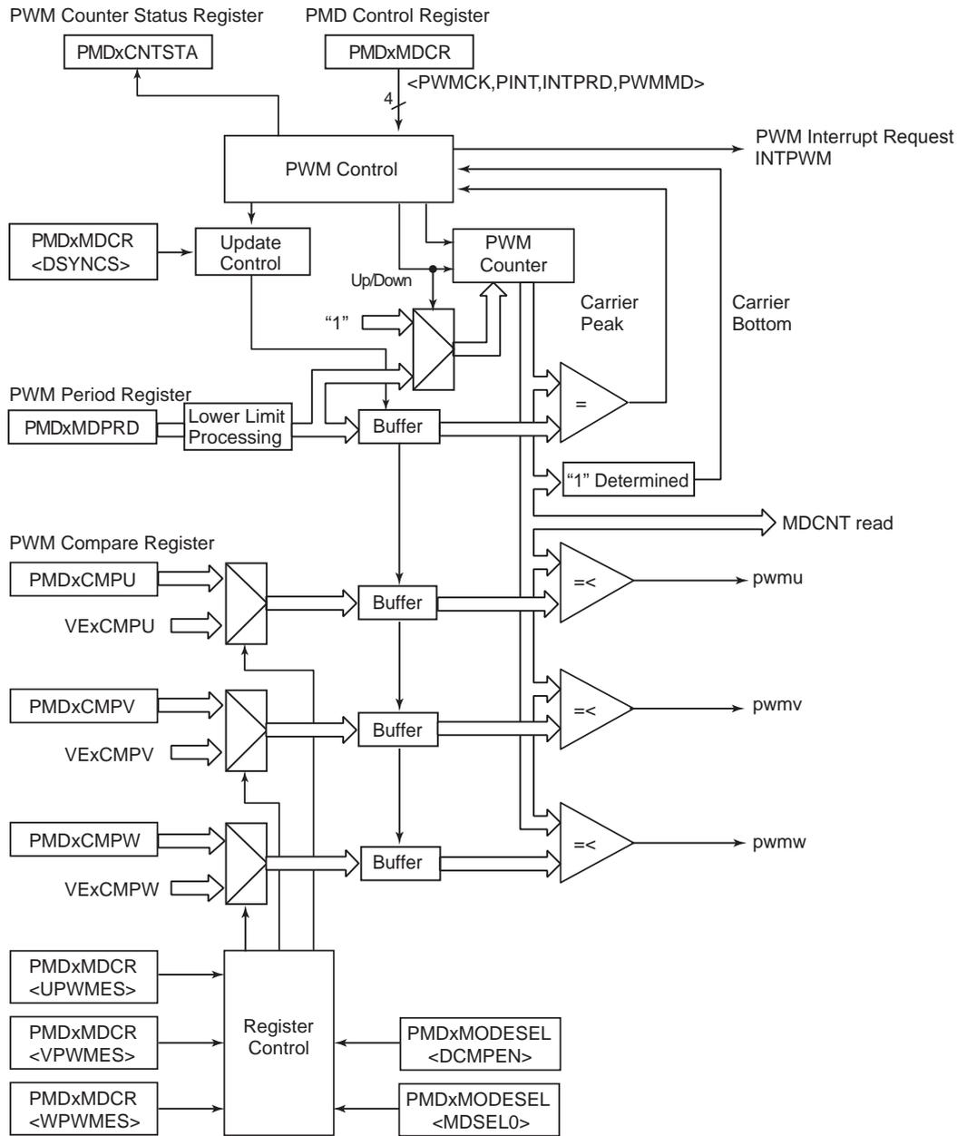
Figure 17-4 Pulse Width Modulation Circuit
