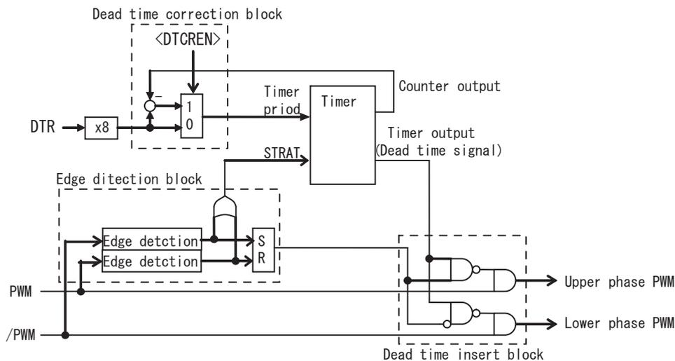
Figure 17-10 The dead time unit configuration
