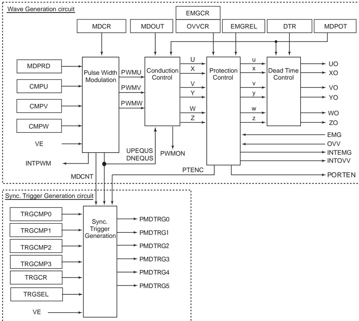
Figure 17-3 Block diagram of PMD Circuit
