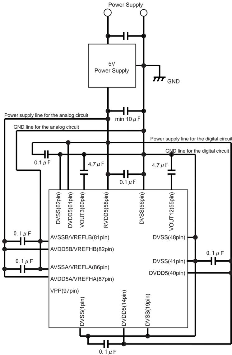
Figure 1-3 Capacitors for power supply pins connection circuit
