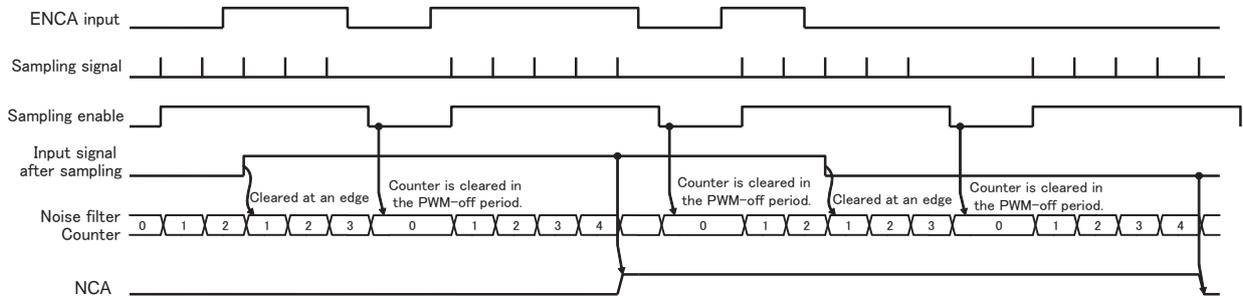
Figure 19-7 Noise cancelling (Sampling in the PWM-on period. Noise cancelling timer is cleared in the PWM-off period.<NCT>=4)
