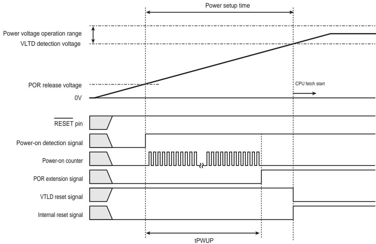
Figure 5-2 Reset Operation by Low-voltage-detection Circuit (not using  $\overline{\text{RESET}}$  pin)
