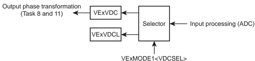
Note) When a power supply voltage controlled by VExVDC register is corrected, select VExVDCL register as a storage location, and set a corrected value in VExDVC register.
