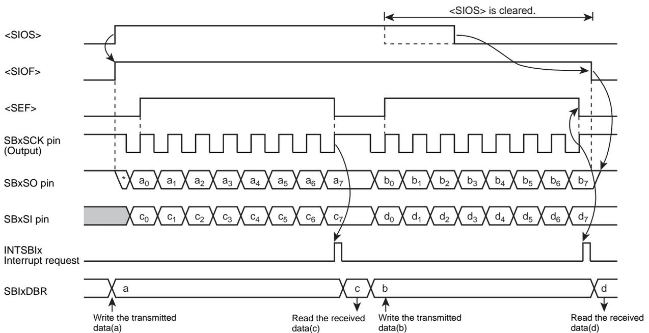
Figure 14-18 Transmit/Receive Mode (Example: Internal Clock)
