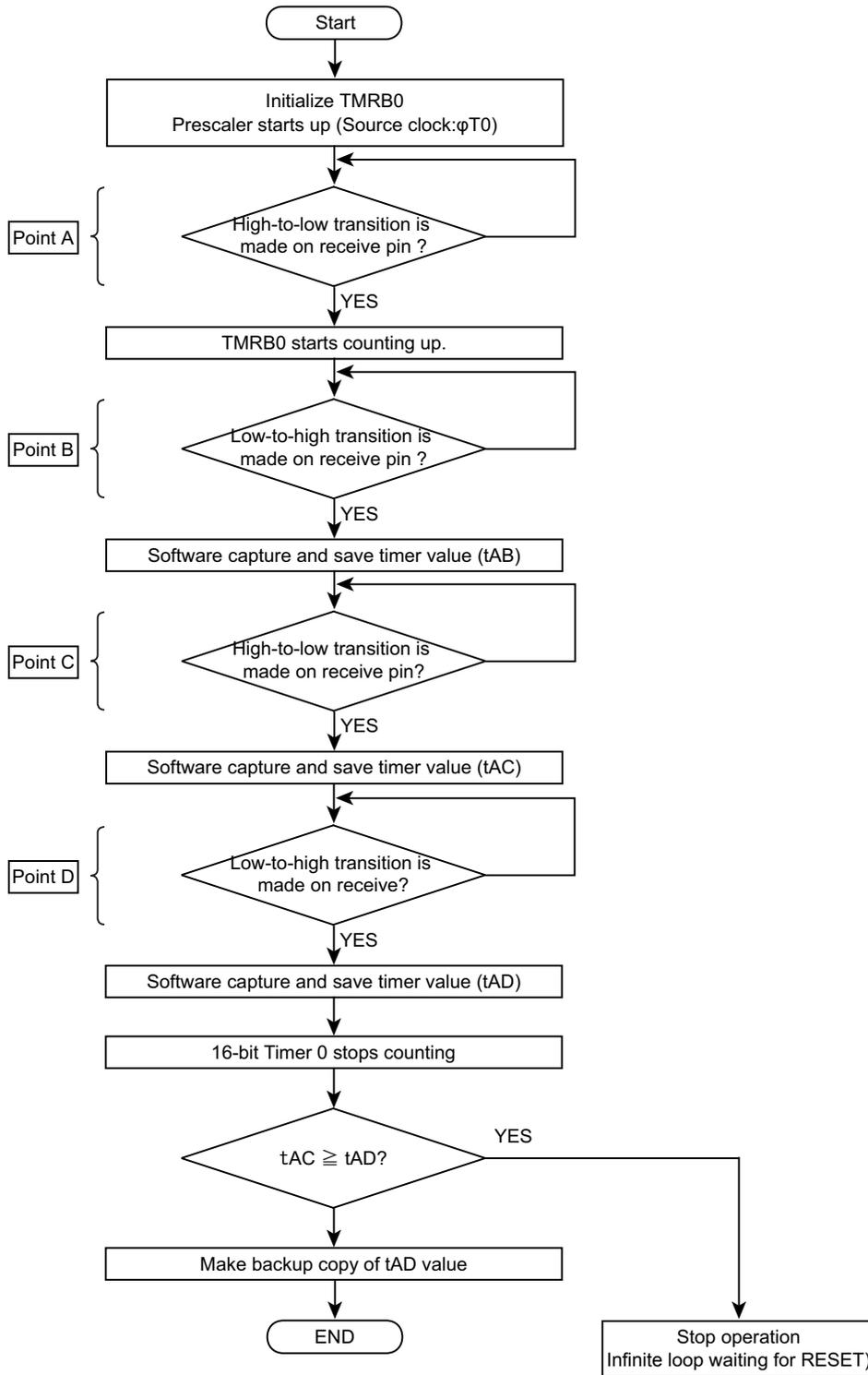
Figure 24-8 Serial operation mode receive flow chart
