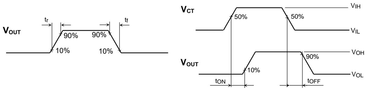
Figure 1 t<sub>r</sub>, t<sub>f</sub>, t<sub>ON</sub>, t<sub>OFF</sub> Waveforms
