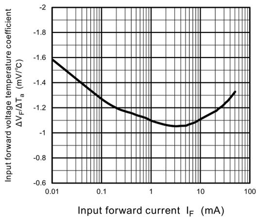
**Fig. 11.5  $\Delta V_F / \Delta T_a - I_F$**
