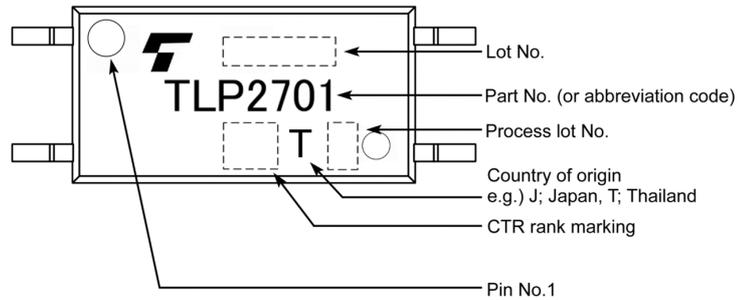
Note: A different marking is used for photocouplers that have been qualified according to option (D4) of EN 60747. See Fig.15.3.
