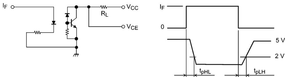
Fig. 10.1 Switching Time Test Circuit and Waveform
