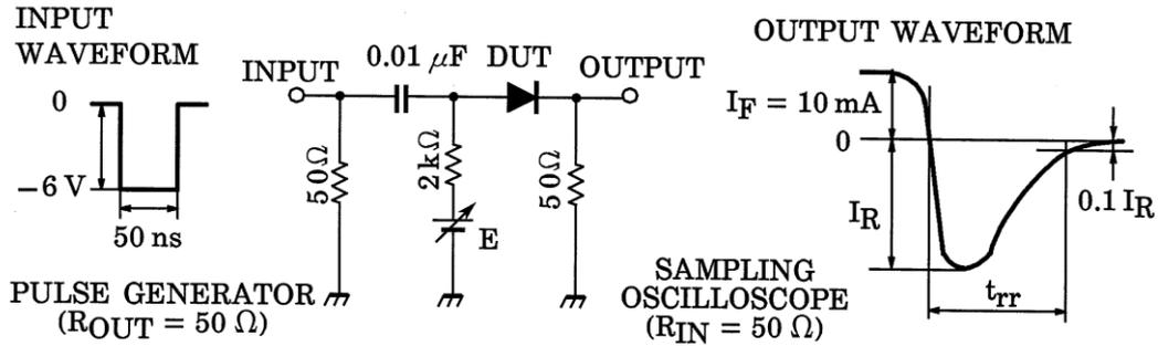
**Fig.1 Reverse Recovery Time ( $t_{rr}$ ) Test Circuit**
