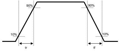
Figure 6.1 Switching characteristics
