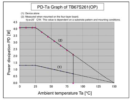
Figure 10.1 Power dissipation
