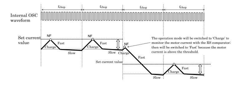
Figure 5.5 ADMD current waveform (When the next current step is lower)
