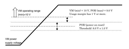
Figure 1.1 Power supply voltage and usage range
