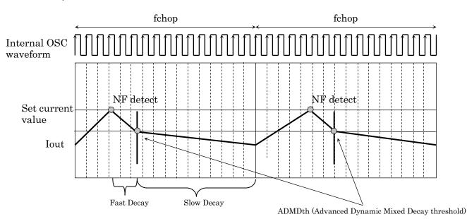
Auto Decay Mode waveform (current waveform)
