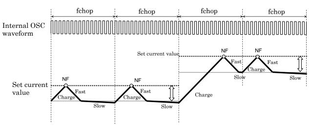
Figure 5.3 ADMD current waveform
