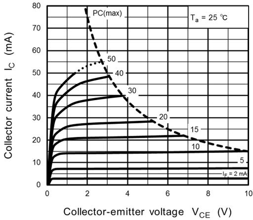
**Fig. 11.7  $I_C - V_{CE}$**
