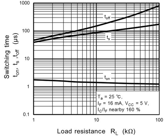
**Fig. 11.14** Switching Time -  $R_L$
