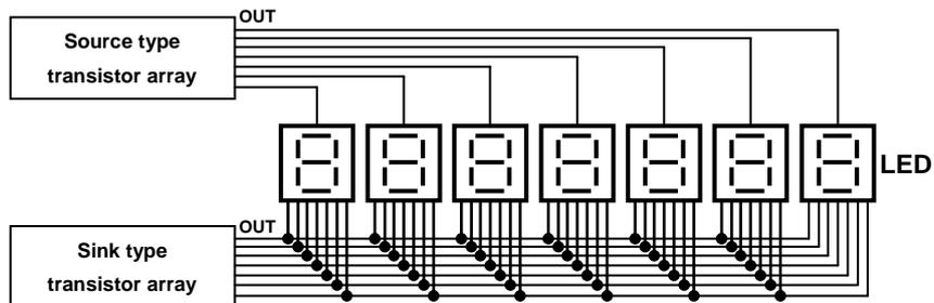
●Construction of output circuit
