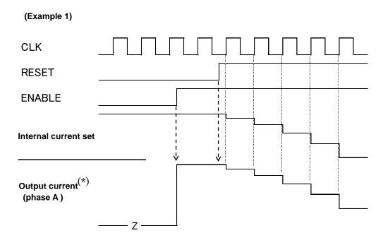
(\*: Output current starts rising at the timing of PWM frequency just after ENABLE pin outputs high.)
