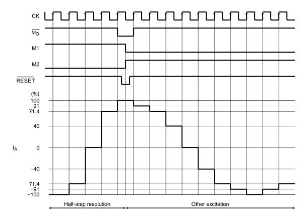
It is recommended that the state of the M1, M2 and M3 pins be changed after setting the  $\overline{RESET}$  signal Low during the Initial state ( $\overline{M_O}$  = Low). Even when the  $\overline{M_O}$  signal is Low, changing the M1, M2 and M3 signals without setting the  $\overline{RESET}$  signal Low may cause a discontinuity in the current waveform.
