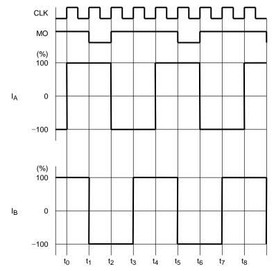
Half-step resolution (A type) (M1: L, M2: H, M3: L, CW Mode)
