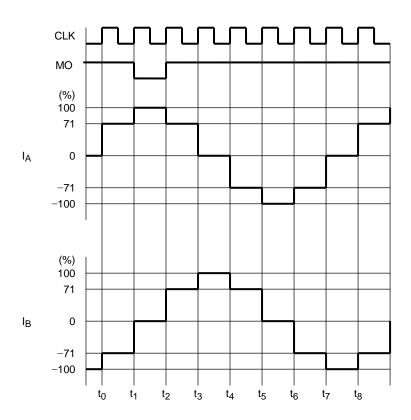
Half-step resolution (A type) (M1: L, M2: H, M3: L, CCW Mode)
