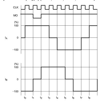
Half-step resolution (B type) (M1: L, M2: H, M3: H, CCW Mode)
