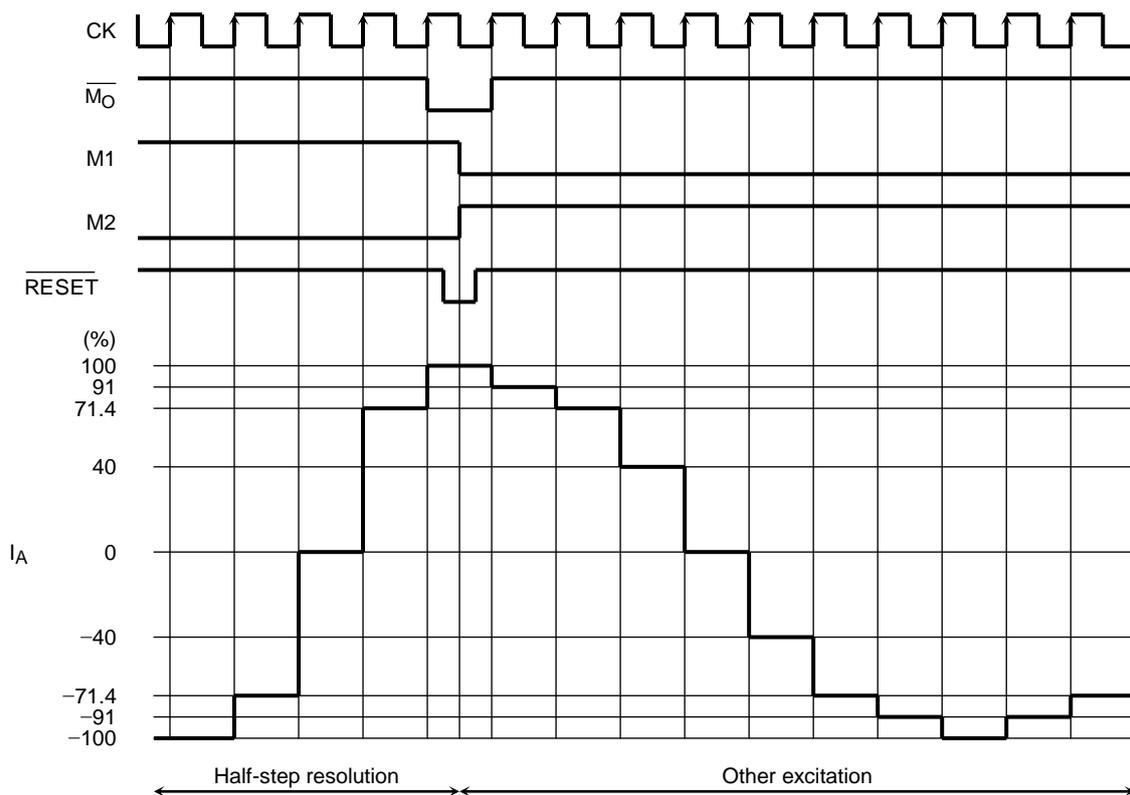
It is recommended that the state of the M1, M2 and M3 pins be changed after setting the  $\overline{\text{RESET}}$  signal Low during the Initial state ( $\overline{\text{M0}} = \text{Low}$ ). Even when the  $\overline{\text{M0}}$  signal is Low, changing the M1, M2 and M3 signals without setting the  $\overline{\text{RESET}}$  signal Low may cause a discontinuity in the current waveform.
