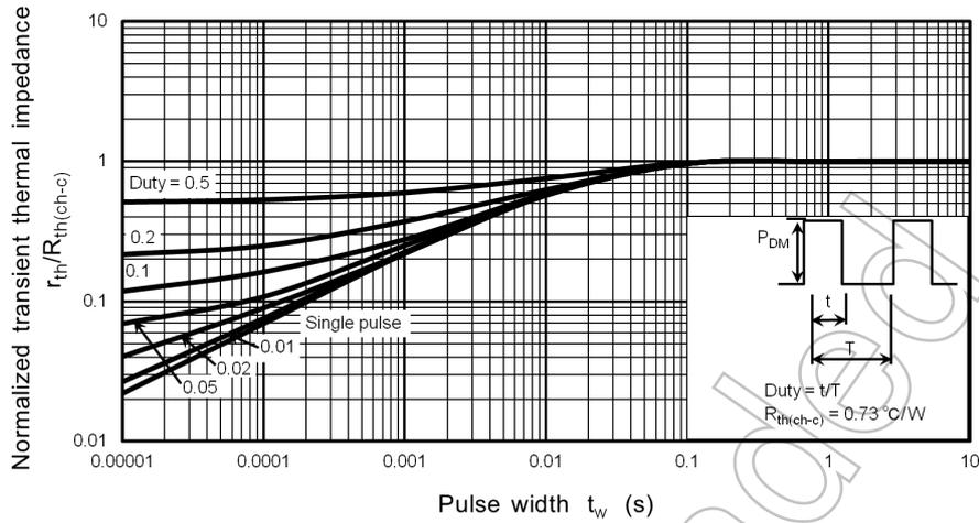
**Fig. 9.13**  $r_{th}/R_{th(ch-c)} - t_w$
