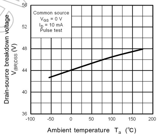
Fig. 9.12  $V_{(BR)DSS} - T_a$
