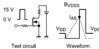
$$R_G = 1 \Omega, V_{DD} = 32 \text{ V}, L = 29 \mu\text{H} \quad E_{AS} = \frac{1}{2} \cdot L \cdot I_{AS}^2 \cdot \left( \frac{B_{VDSS}}{B_{VDSS} - V_{DD}} \right)$$
