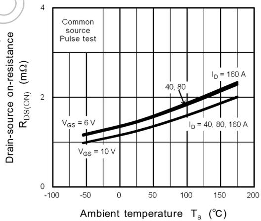
Fig. 9.6  $R_{DS(ON)} - T_a$
