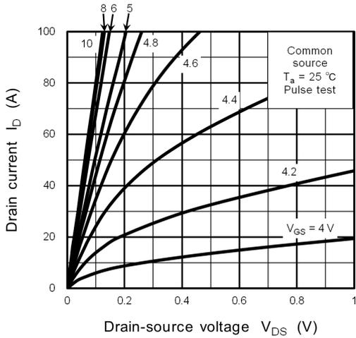
Fig. 9.1  $I_D - V_{DS}$
