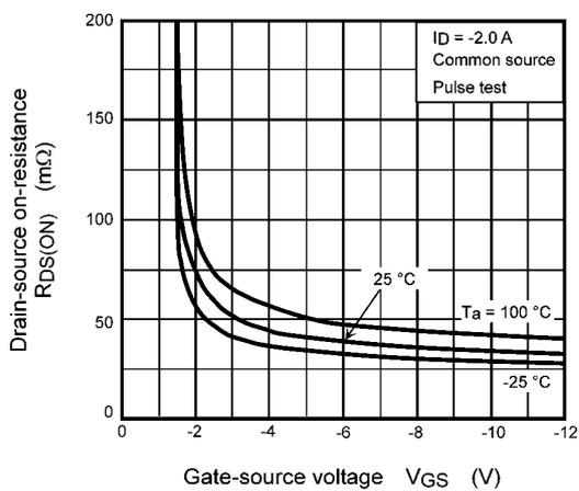
**Fig. 9.2.3**  $R_{DS(ON)} - V_{GS}$
