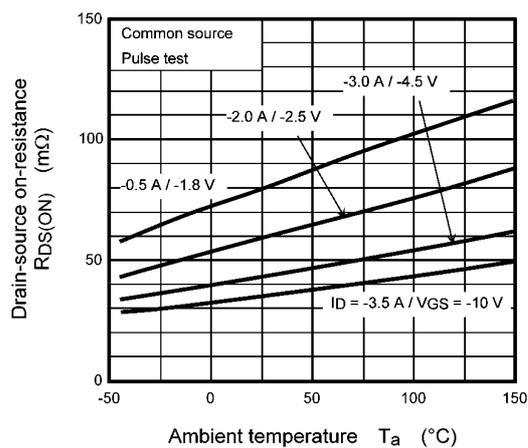
**Fig. 9.2.5**  $R_{DS(ON)} - T_a$
