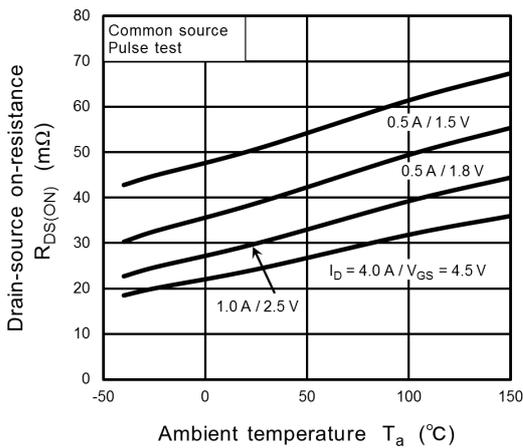
**Fig. 9.1.5**  $R_{DS(ON)} - T_a$
