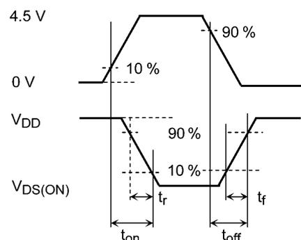
Input Waveform/Output Waveform
