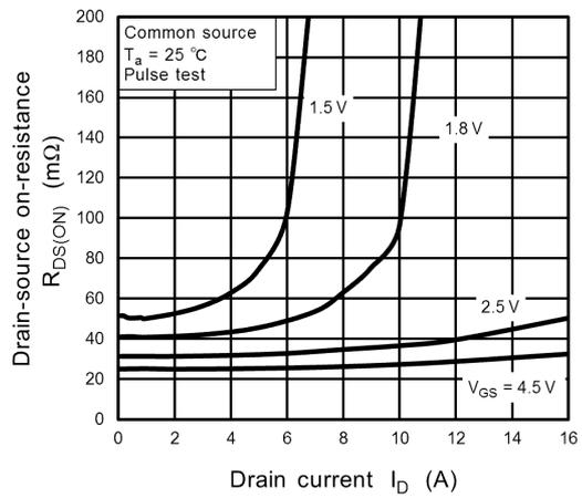
**Fig. 9.1.4**  $R_{DS(ON)} - I_D$
