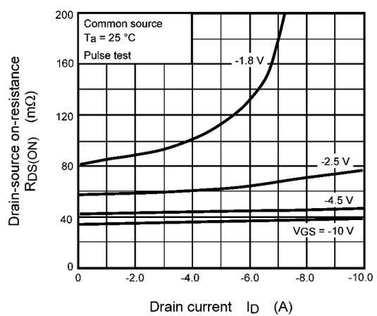
**Fig. 9.2.4**  $R_{DS(ON)} - I_D$
