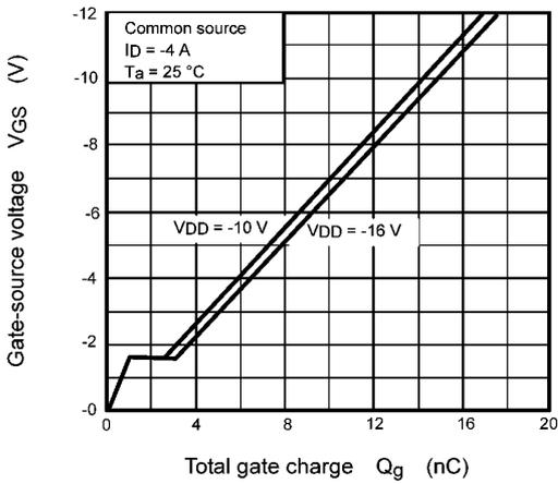
**Fig. 9.2.9 Dynamic Input Characteristics**
