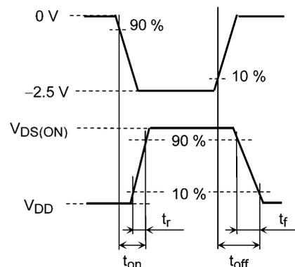
Input Waveform/Output Waveform
