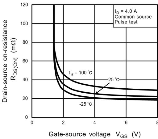
**Fig. 9.1.3**  $R_{DS(ON)} - V_{GS}$
