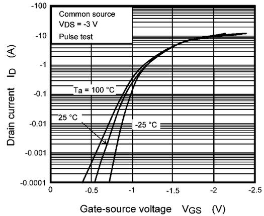
**Fig. 9.2.2**  $I_D - V_{GS}$
