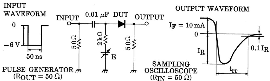
**Fig.1 Reverse Recovery Time (t<sub>rr</sub>) Test Circuit**
