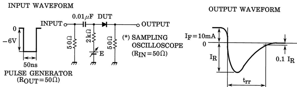
Fig.1 Reverse Recovery Time (t<sub>rr</sub>) Test Circuit
