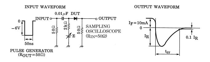
Fig.1 Reverse recovery time (trr) test circuit
