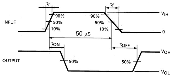
Note 1: Pulse width 50 μs, Duty cycle 10%
