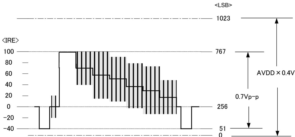
CVBS(Y) signal (10bit ADC) has to input 0.7 Vp-p (equal 140IRE) when input signal is NTSC.
