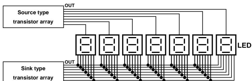
●Construction of output circuit
