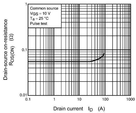
Fig. 8.6  $R_{DS(ON)} - I_D$
