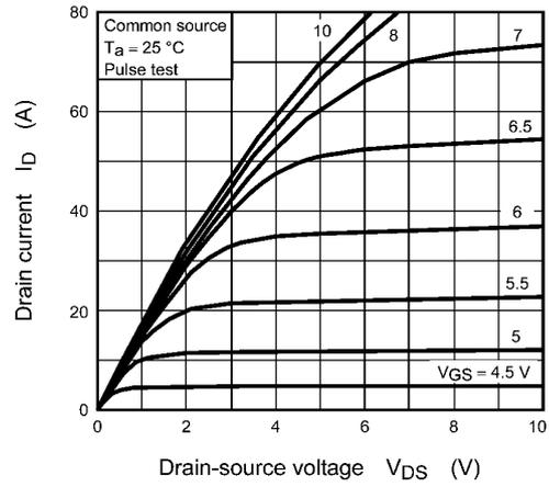
Fig. 8.2  $I_D - V_{DS}$
