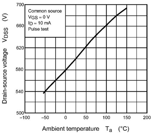
Fig. 8.5  $V_{DSS} - T_a$
