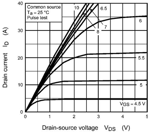
Fig. 8.1  $I_D - V_{DS}$
