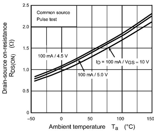
**Fig. 8.5**  $R_{DS(ON)} - T_a$
