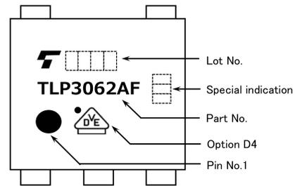
**Fig. 16.4 Marking Example of TLP 3062AF (Note)**
